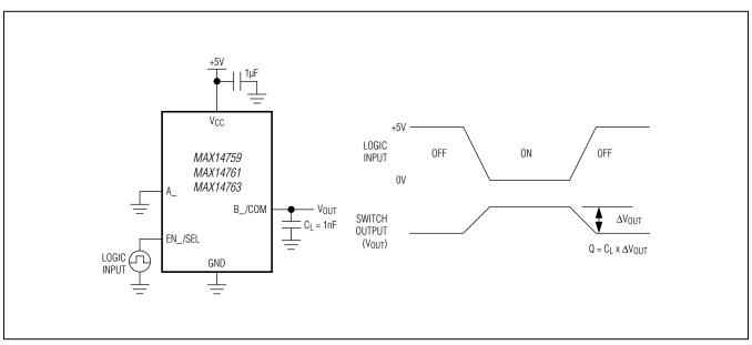
Figure 7. Charge Injection
