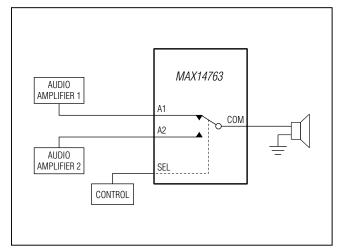
Figure 13. Single-Ended Amplifier Switching
