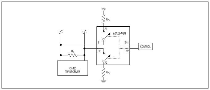
Figure 11. Pullup and Pulldown Resistance Switch
