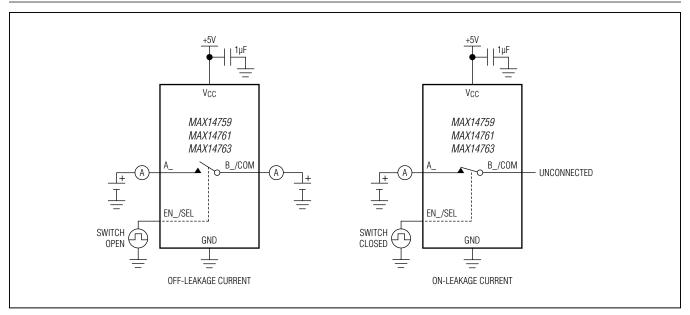
Figure 1. Leakage Current Measurement
