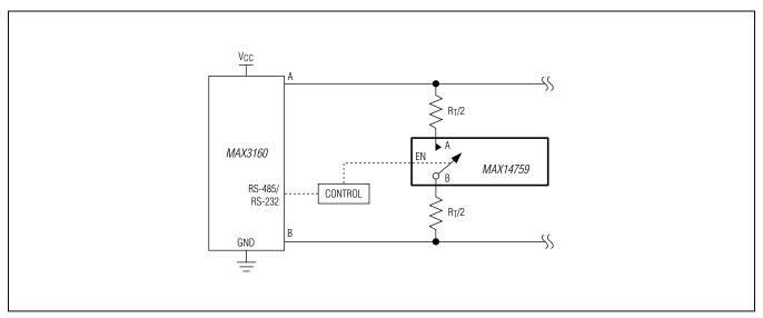
Figure 10. Multiprotocol Termination Switch
