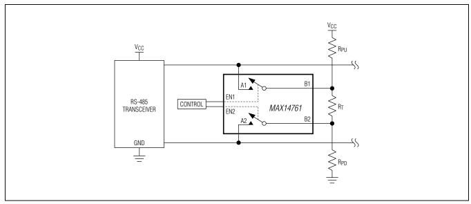
Figure 12. Fail-Safe Biasing Network Switch
