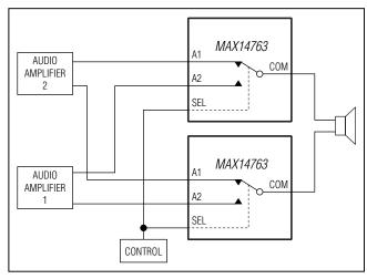
Figure 14. Differential Amplifier Switching
