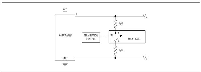
Figure 8. RS-485 Termination Switch
