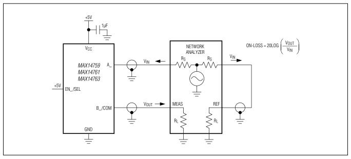
Figure 6. Insertion Loss
