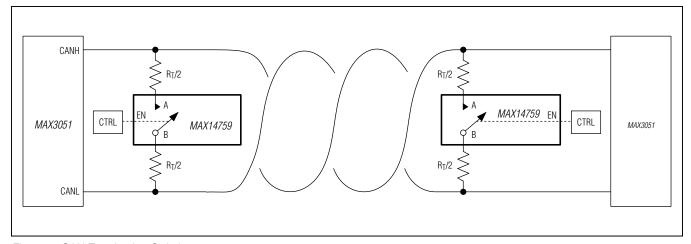
Figure 9. CAN Termination Switch
