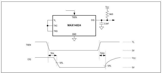
Figure 2. Driver Enable Low and Disable High Timing
