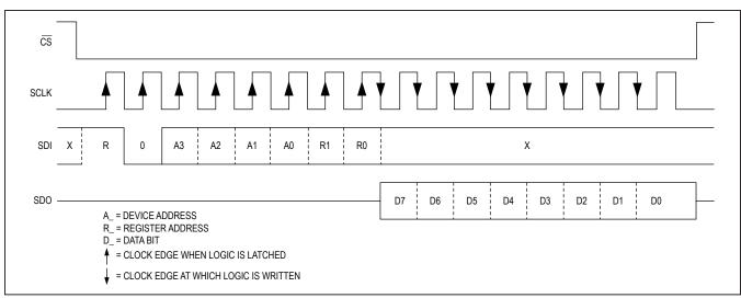
Figure 9. SPI Read Cycle
