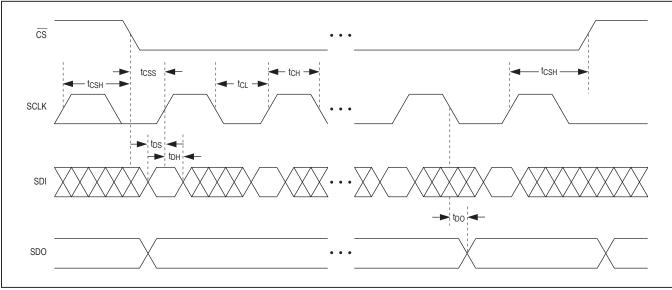
Figure 6. SPI Timing Diagram
