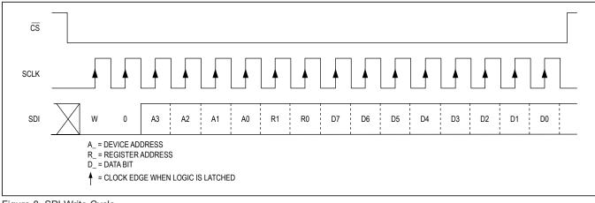
Figure 8. SPI Write Cycle
