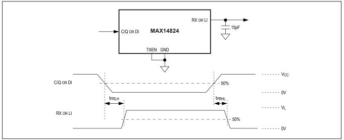
Figure 4. Receiver Polarity and Timing
