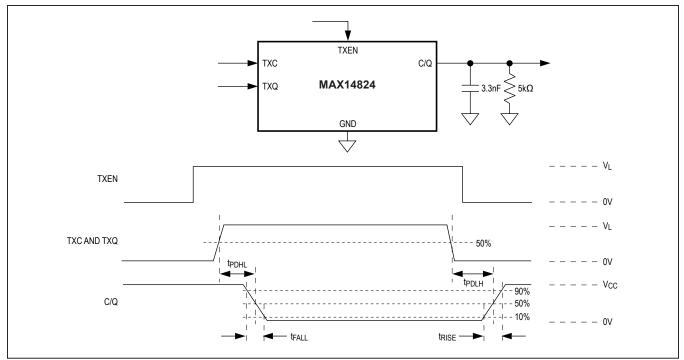
Figure 1. Driver Polarity and Timing
