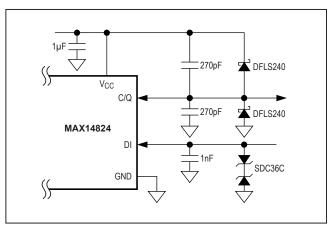
Figure 11. MAX14824 Operating Circuit with TVS Protection
