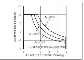
Figure 1. Maximum Output Current Curves
