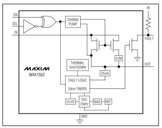
the MAX1562/MAX1562H and 1.35W for the MAX1563, the devices' die temperature exceeds the +160°C thermal-shutdown threshold, and the switch output shuts down until the junction temperature cools by 15°C. The duty cycle and period are strong functions of the ambient temperature and the PC board layout.
