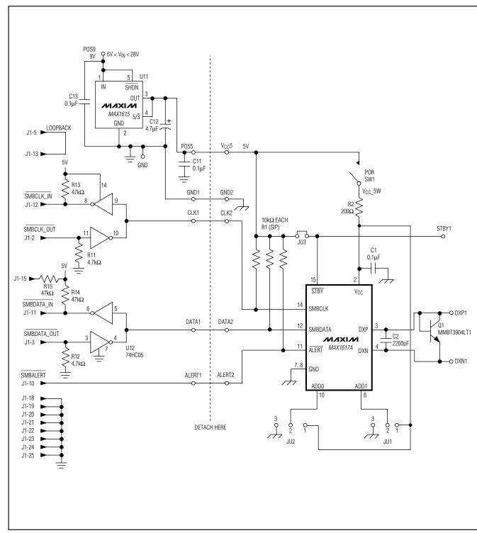
Figure 1. MAX1617A EV Kit Schematic
