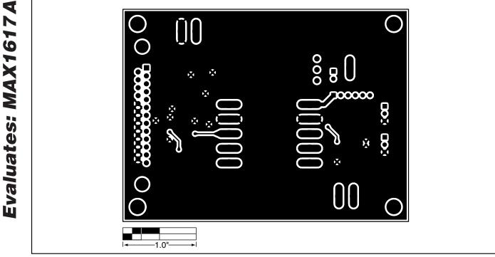
Figure 4. MAX1617A EV Kit PC Board Layout—Solder Side
