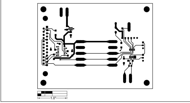
Figure 3. MAX1617A EV Kit PC Board Layout—Component Side
