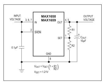
Figure 3. Adjustable Output Configuration Using External Feedback Resistors
