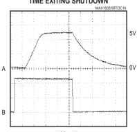
A: OUTPUT VOLTAGE (2V/div) B: SHDN PIN VOLTAGE (2V/div)
