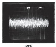
10Hz TO 100kHz NOISE, V<sub>OUT</sub> = 5V (1mV/div), I<sub>OUT</sub> = 165mA
