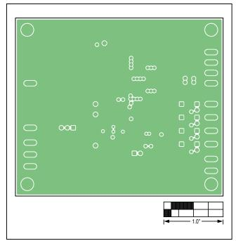
Figure 5. MAX16813 EV Kit PCB Layout—PGND Layer 3
