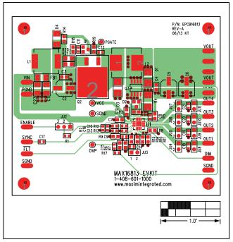
Figure 3. MAX16813 EV Kit PCB Layout—Component Side
