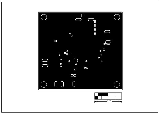
Figure 4. MAX16834 EV Kit PCB Layout—GND Layer 2
