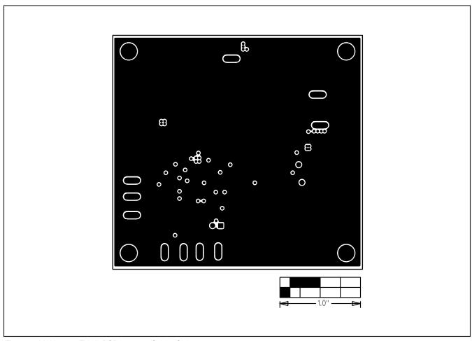
Figure 6. MAX16834 EV Kit PCB Layout—Solder Side
