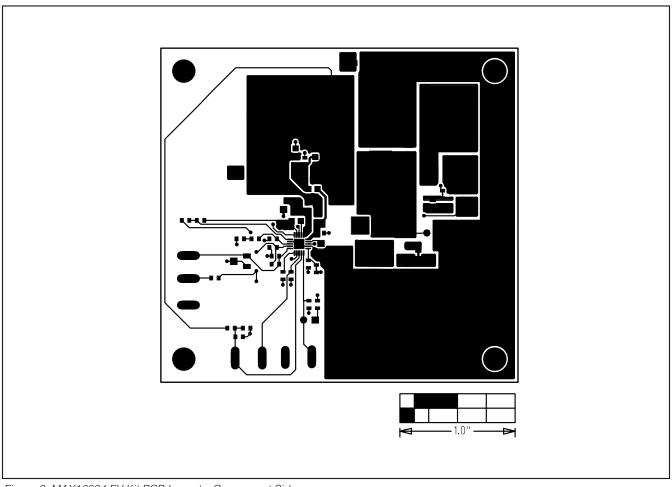
Figure 3. MAX16834 EV Kit PCB Layout—Component Side
