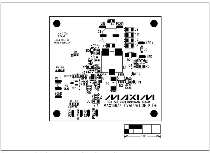
Figure 2. MAX16834 EV Kit Component Placement Guide—Component Side
