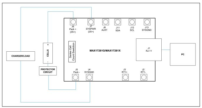
Figure 1. MAX17261 Board Connections
