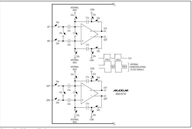
Figure 1. Rx ADC Internal T/H Circuits
