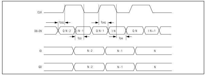
Figure 5. Tx DAC System Timing Diagram
