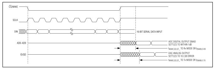
Figure 7. Mode-Recovery Timing Diagram
