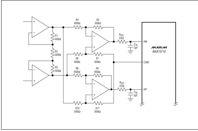
Figure 12. Rx ADC DC-Coupled Differential Drive
