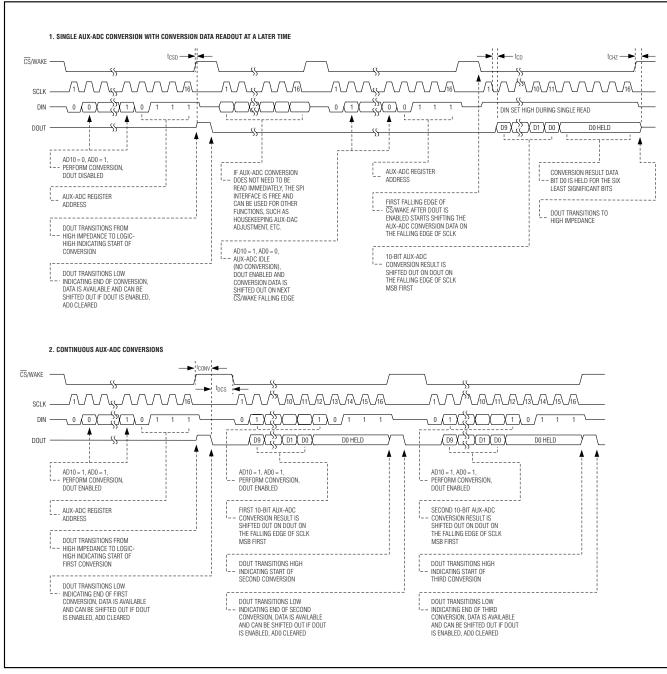
Figure 8. Aux-ADC Conversions Timing
