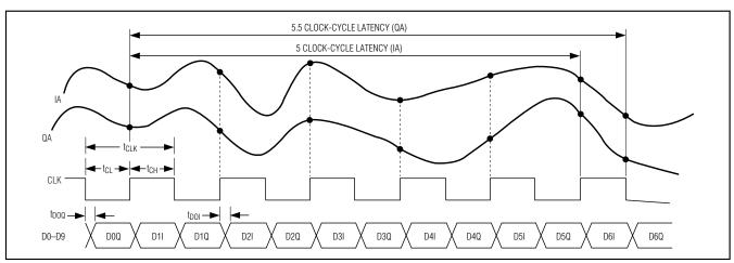
Figure 3. Rx ADC System Timing Diagram
