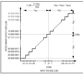
Figure 2. Rx ADC Transfer Function
