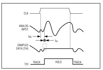
Figure 15. T/H Aperture Timing
