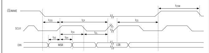
Figure 6. Serial-Interface Timing Diagram
