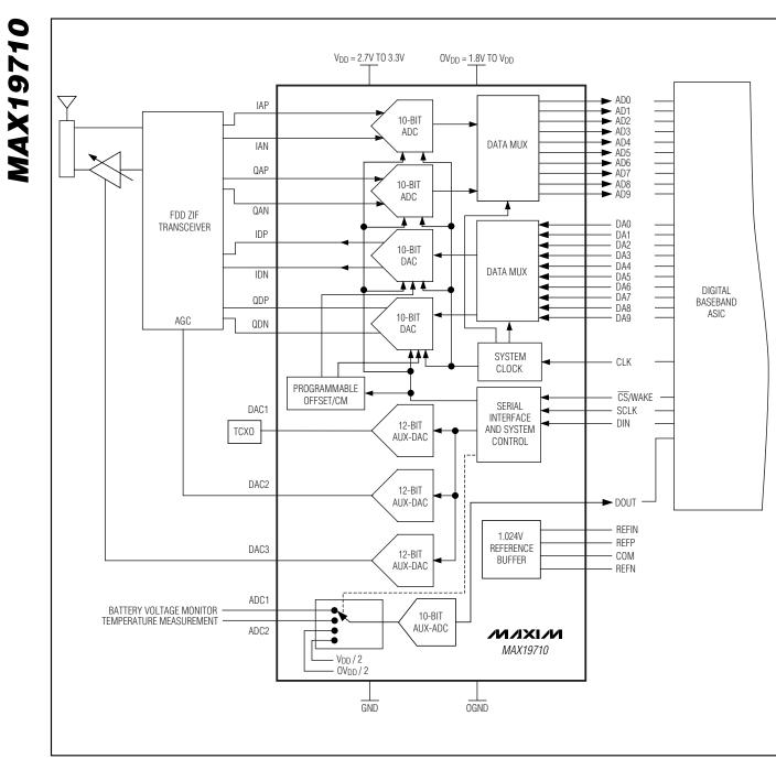
Figure 13. Typical FDD Application Circuit
