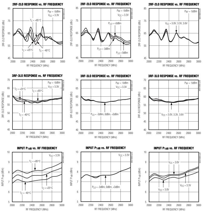
(Typical Application Circuit, Vcc = +3.3V, PLO = 0dBm, PRF = -5dBm, LO is low-side injected for a 300MHz IF, T<sub>C</sub> = +25°C, unless
