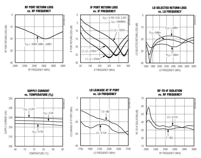
(Typical Application Circuit, Vcc = +3.3V, PLO = 0dBm, PRF = -5dBm, LO is low-side injected for a 300MHz IF, T<sub>C</sub> = +25°C, unless
