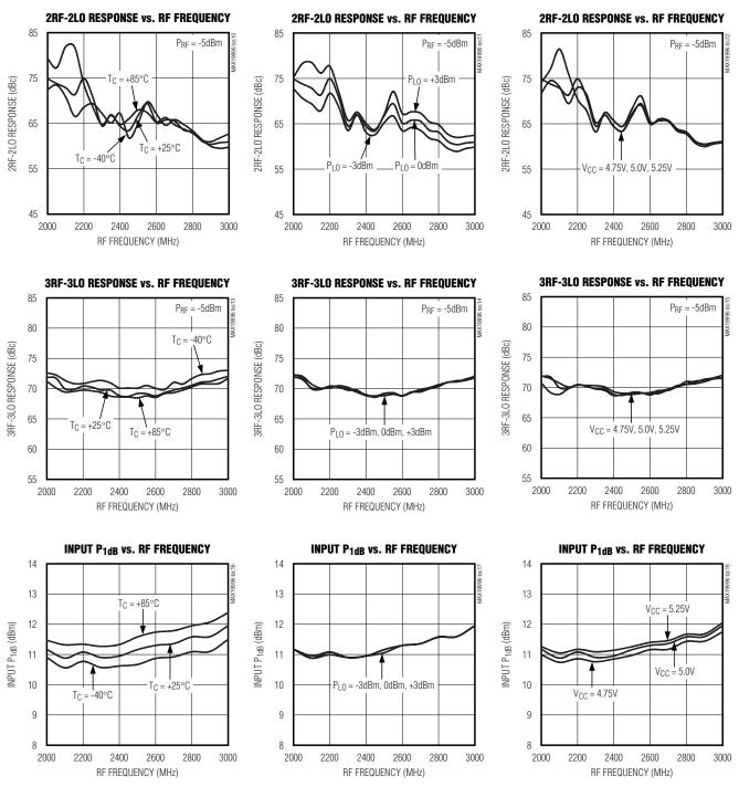
(Typical Application Circuit, Vcc = +5.0V, PLO = 0dBm, PRF = -5dBm, LO is low-side injected for a 300MHz IF, Tc = +25°C, unless
