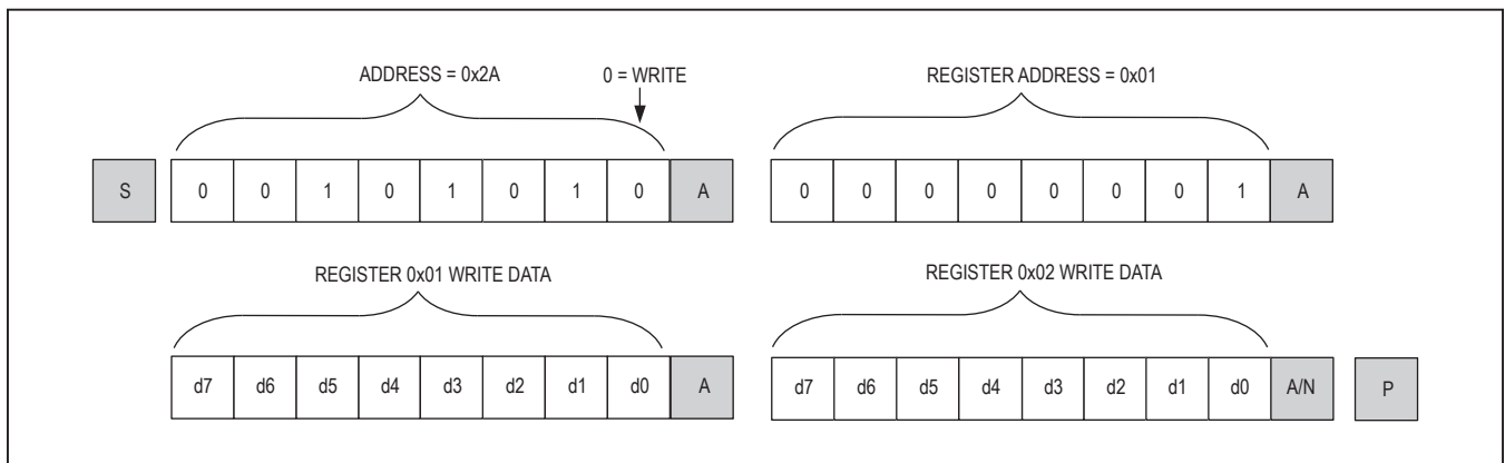
Figure 8. Format for Writing to Multiple Registers
