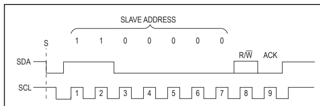
Figure 1. MAX2112 Slave Address Byte with ADDR Pin Connected to Ground
