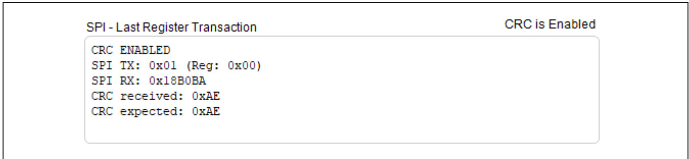
Figure 5. SPI Read Transaction with CRC Enabled
