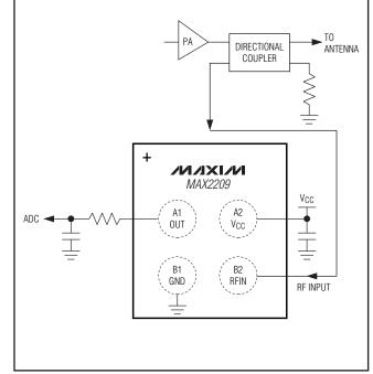
Figure 1. Typical Application Circuit
