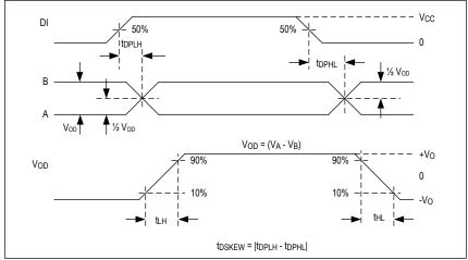
Figure 3. Driver Propagation Delays
