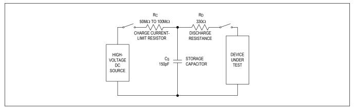
Figure 12. IEC 61000-4-2 ESD Test Model
