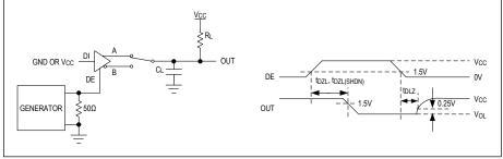
Figure 5. Driver Enable and Disable Times (t<sub>DZL</sub>, t<sub>DLZ</sub>)
