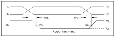
Figure 7. Receiver Propagation Delays
