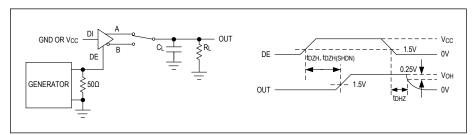
Figure 4. Driver Enable and Disable Times (t<sub>DZH</sub>, t<sub>DHZ</sub>)
