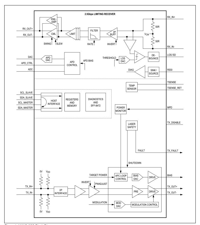
Figure 1. MAX24002 Block Diagram
