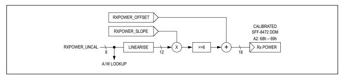
Figure 15. Calculating the Rx Power DDM
