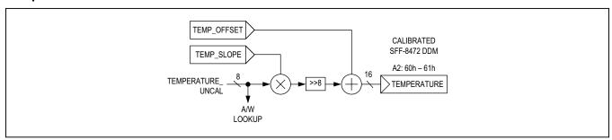
Figure 11. Calculating the Temperature DDM
