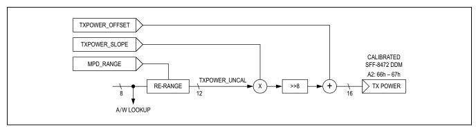
Figure 14. Calculating the Tx Power DDM
