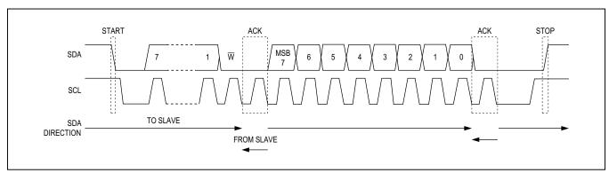
Figure 22. Write Transaction
