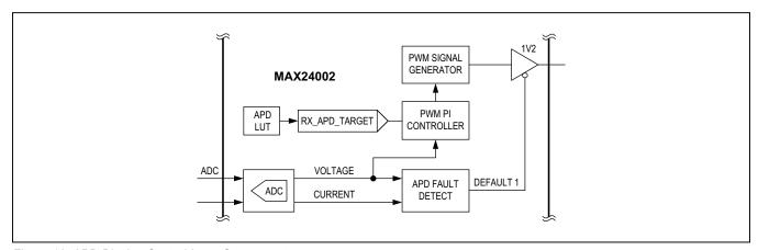
Figure 10. APD Biasing Control Loop Components
