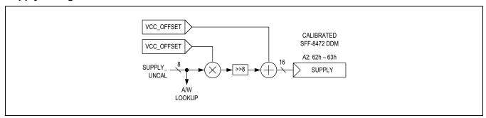
Figure 12. Calculating the Supply Voltage DDM
