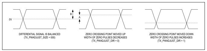
Figure 6. Crossing Point Adjustment
