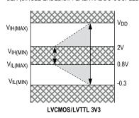
Typical I/O ranges for TX\_IN are shown
