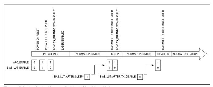
Figure 7. Behavior of the tx\_biasmode Register in Closed-Loop Mode
