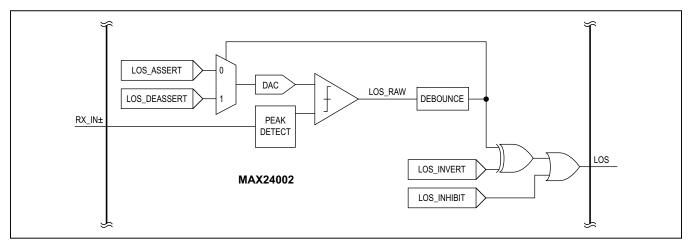
Figure 3. LOS Detection System
