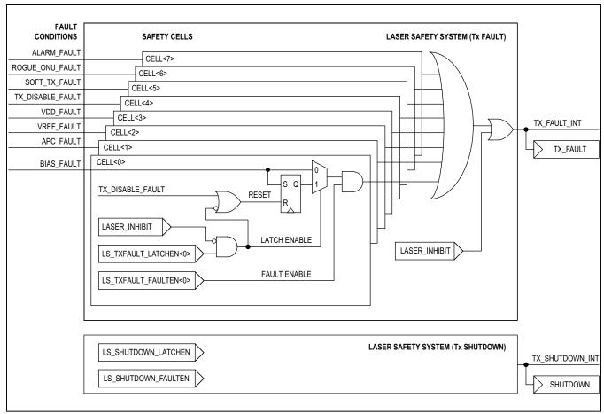
Figure 8. Laser Safety System
