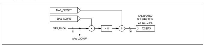
Figure 13. Calculating the Bias Current DDM
