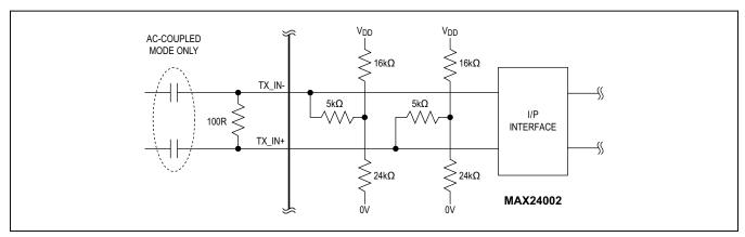
Figure 5. TX\_IN Input Termination and Signal Conditioning
