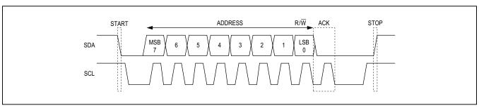
Figure 21. Address Decoding Example
