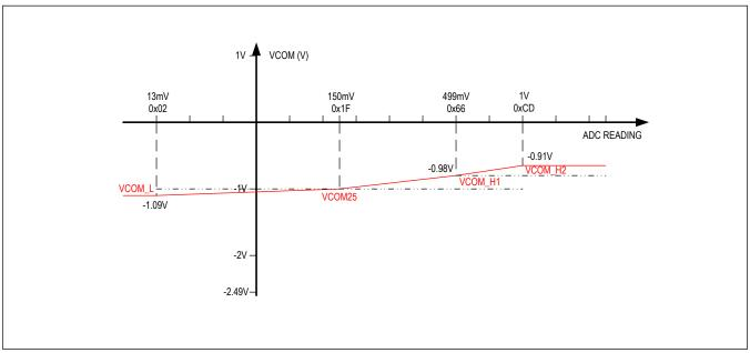
Figure 5. Sample VCOM Temperature Compensation Curve
