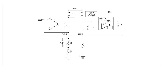
Figure 2. Possible NTC Connection
