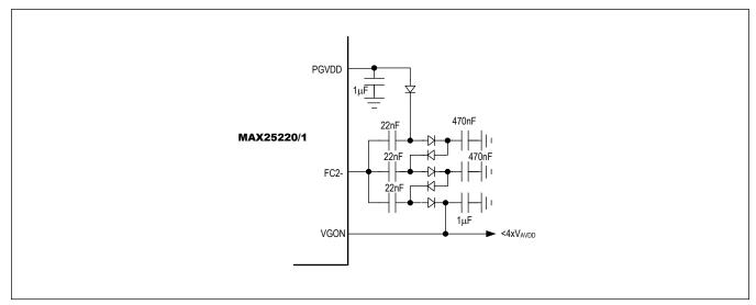
Figure 4. Quadrupler Charge-Pump at 2.1MHz
