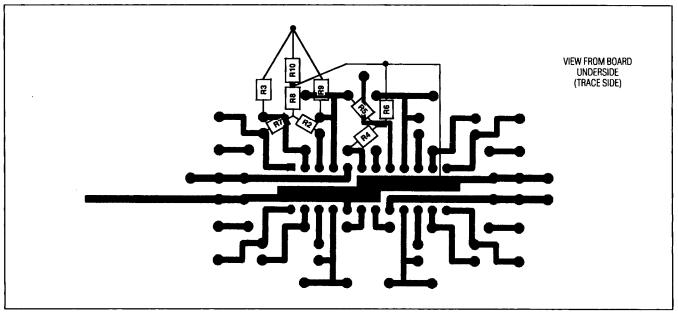
Figure 3. T-Network PC Board Connections
