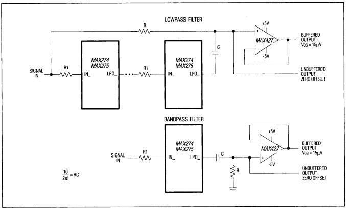
Figure 8b. Trimless Offset Removal
