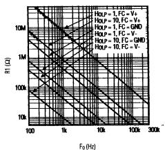
• • • USE RESISTOR "T-NETWORK" TO REDUCE VALUE (SEE HIGH-VALUE RESISTOR TRANSFORMATION SECTION)
