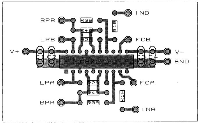
Figure 7b. MAX275 Suggested PC-Board Layout for DIP
