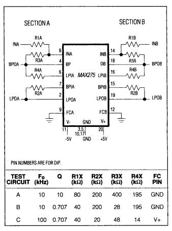
Figure 1b. MAX275 Connection Diagram and Test Circuit
