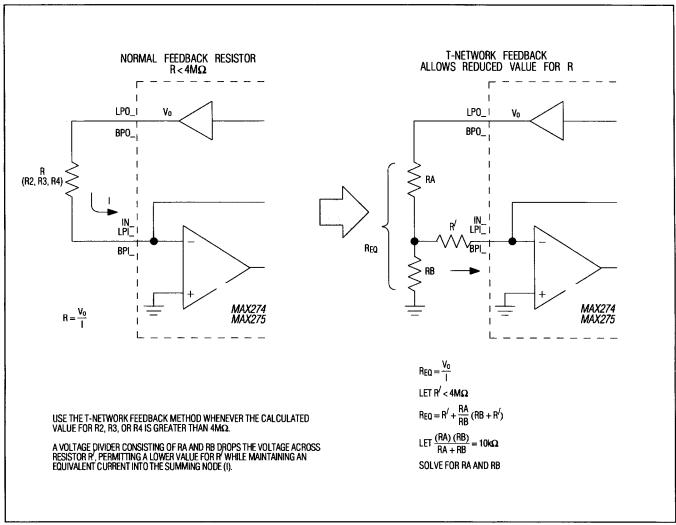
Figure 5. Resistor T-Networks Reduce Resistor Values
