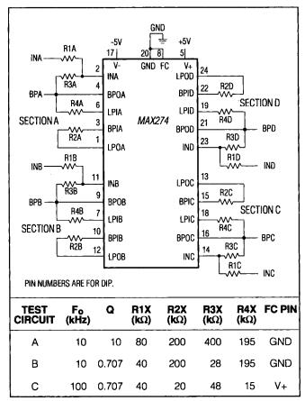
Figure 1a. MAX274 Connection Diagram and Test Circuit
