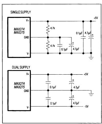
Figure 9. Power-Supply Configurations
