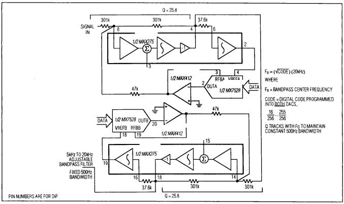
Figure 12. Programmable Bandpass Filter (MAX275)
