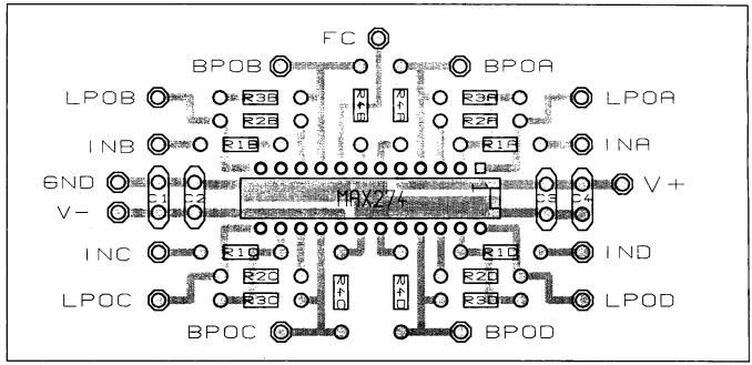
Figure 7a. MAX274 Suggested PC-Board Layout for DIP
