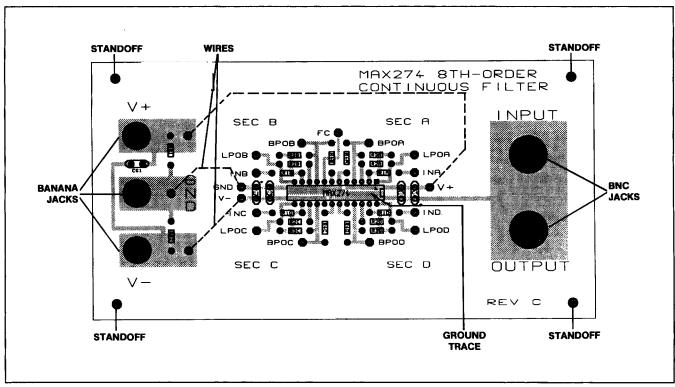
Figure 2. MAX274 EV Kit Component Placement Diagram
