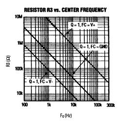
••• USE RESISTOR "T-NETWORK" TO REDUCE VALUE (SEE HIGH-VALUE RESISTOR TRANSFORMATION SECTION)
