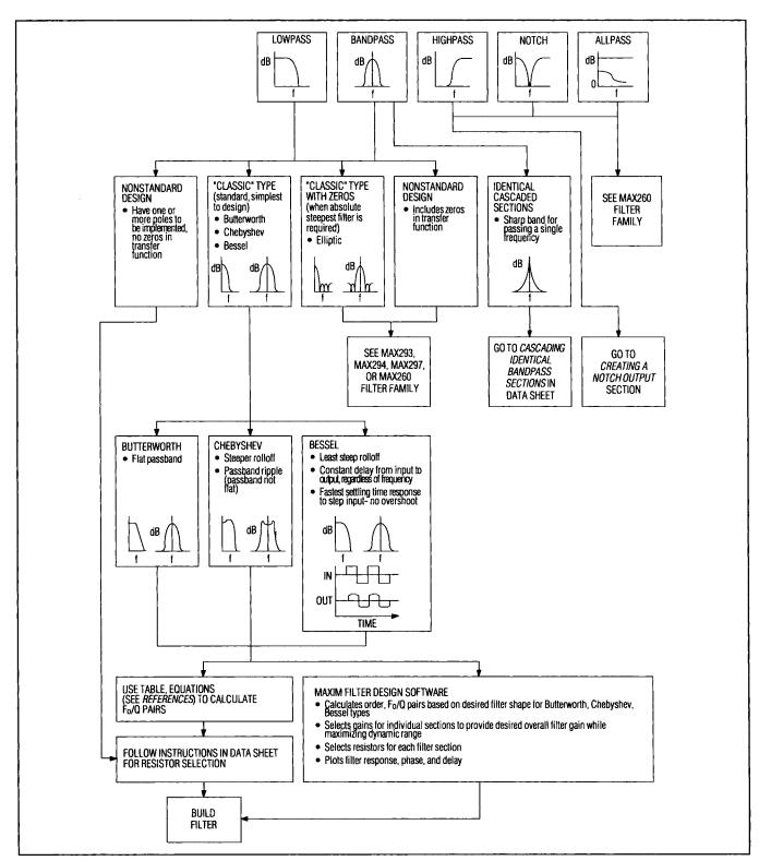
Figure 3. General Filter Design Flowchart
