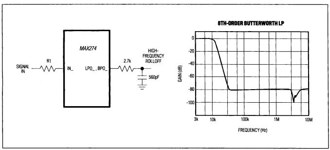
Figure 10. External RC Lowpass for High-Frequency Rolloff
