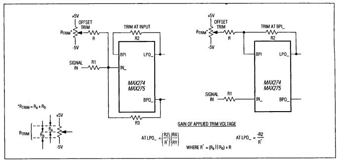
Figure 8a. Trimmed Offset Removal
