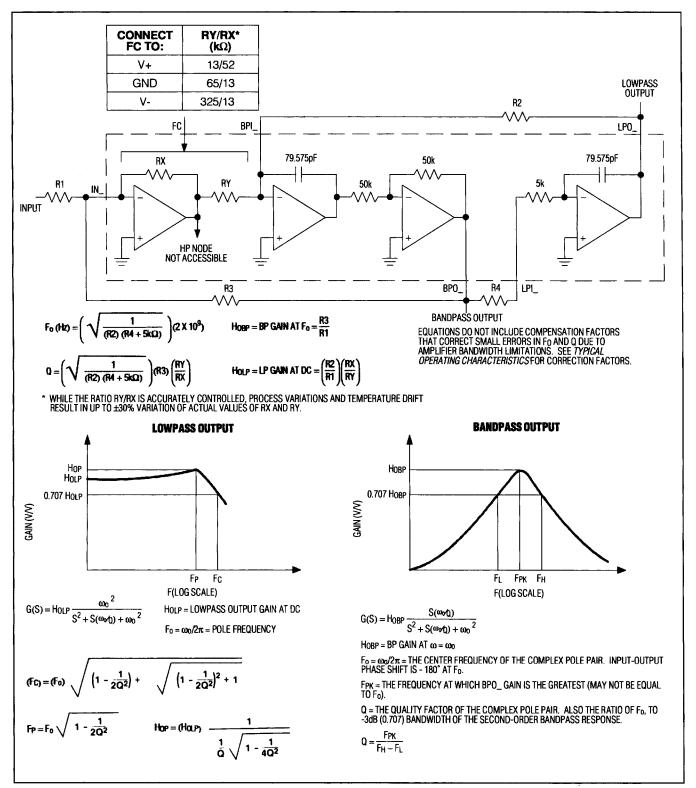
Figure 2. Single 2nd-Order Filter Section
