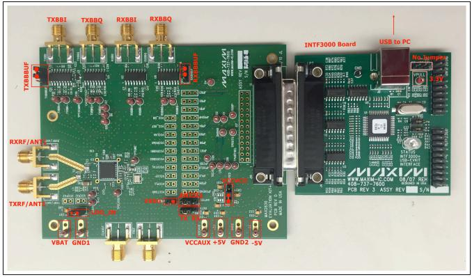
Figure 1. MAX2830 EV Kit Connections
