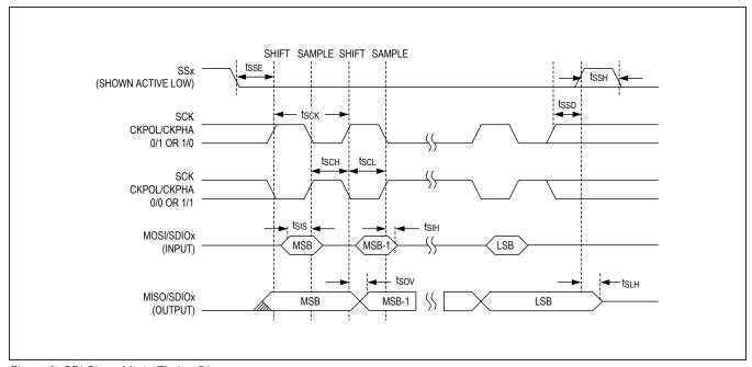
Figure 3. SPI Slave Mode Timing Diagram
