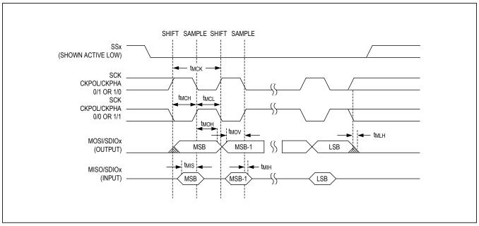
Figure 2. SPI Master Mode Timing Diagram
