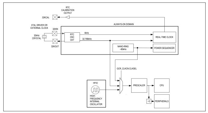
Figure 6. System Clocking Diagram
