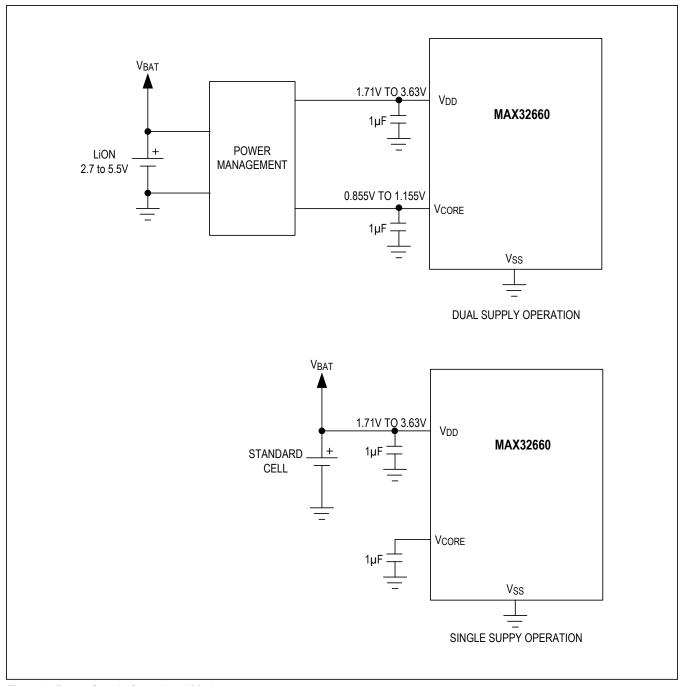
Figure 1. Power Supply Operational Modes
