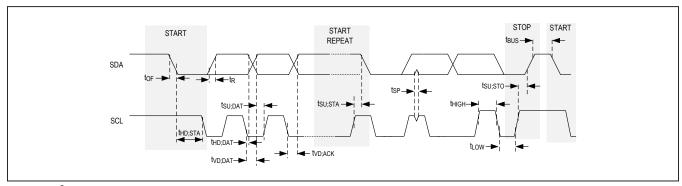
Figure 4. I<sup>2</sup>C Timing Diagram
