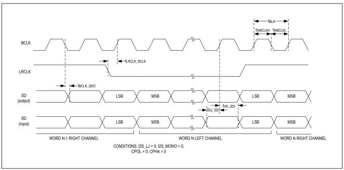
Figure 5. I<sup>2</sup>S Timing Diagram
