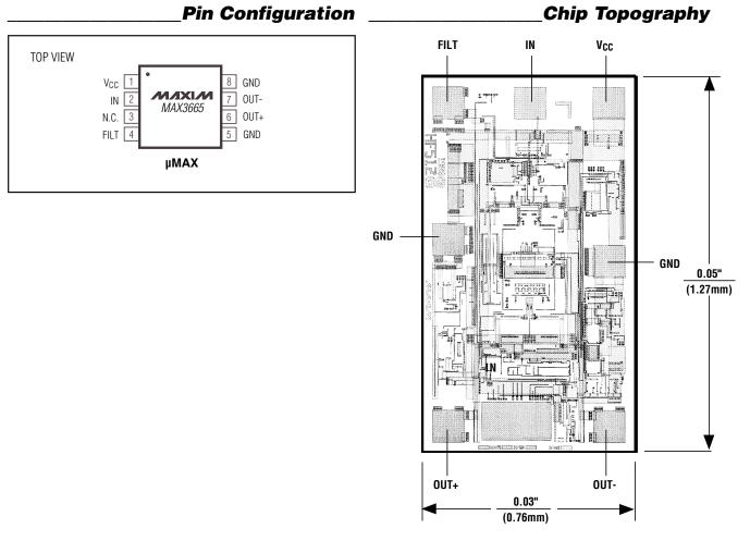
TRANSISTOR COUNT: 443 SUBSTRATE CONNECTED TO GND **MAX3665**
