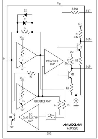
Figure 1. Functional Diagram
