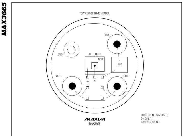
Figure 4. Suggested Layout for TO-46 Header
