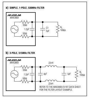
Figure 3. Filter Design Examples
