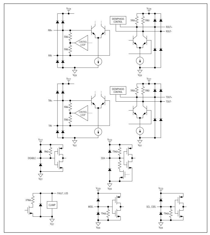
Figure 5. Simplified I/O Structures
