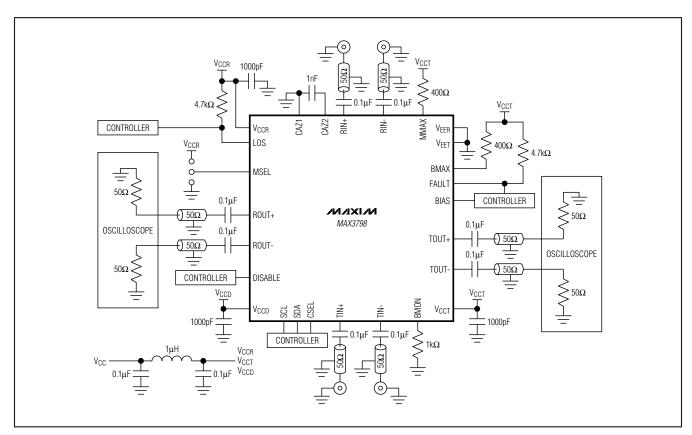
Figure 1. Test Circuit for VCSEL Driver Characterization
