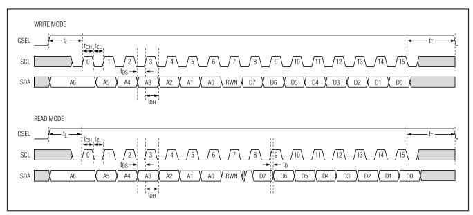
Figure 4. Timing for 3-Wire Digital Interface
