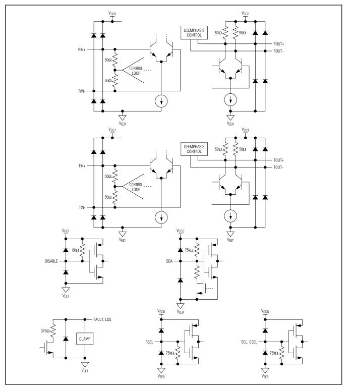
Figure 5. Simplified I/O Structures
