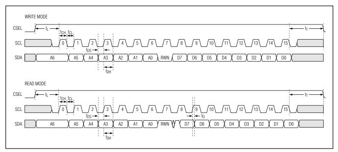
Figure 4. Timing for 3-Wire Digital Interface
