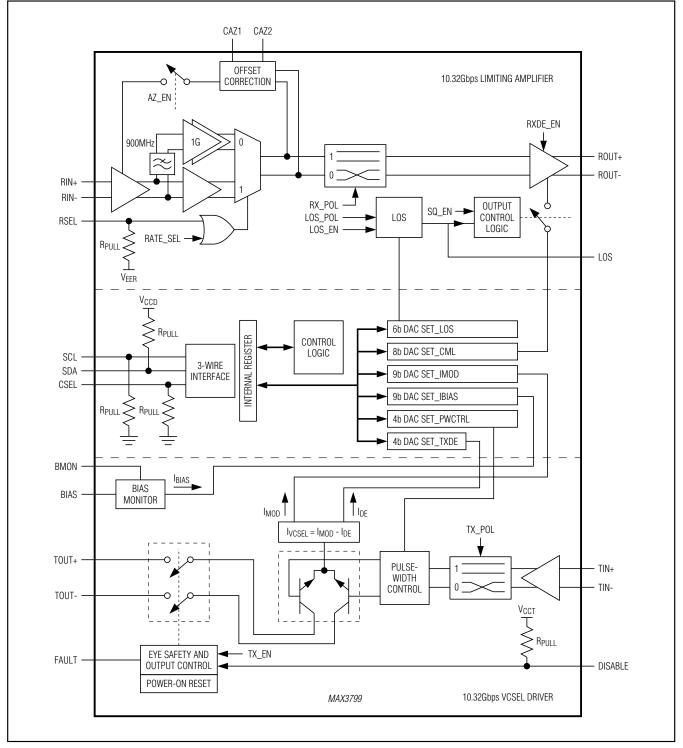
Figure 2. Functional Diagram
