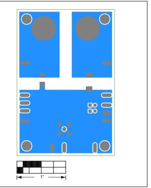
MAX40056 EV Kit PCB Layout Diagrams—Bottom
