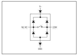
Figure 1. Overvoltage Protection Using External Blocking Diodes
