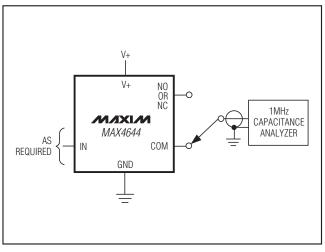
Figure 5. NO, NC, and COM Capacitance
