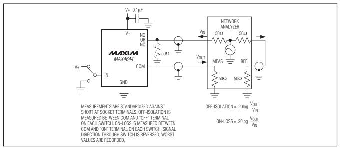
Figure 3. Off-Isolation and On-Loss
