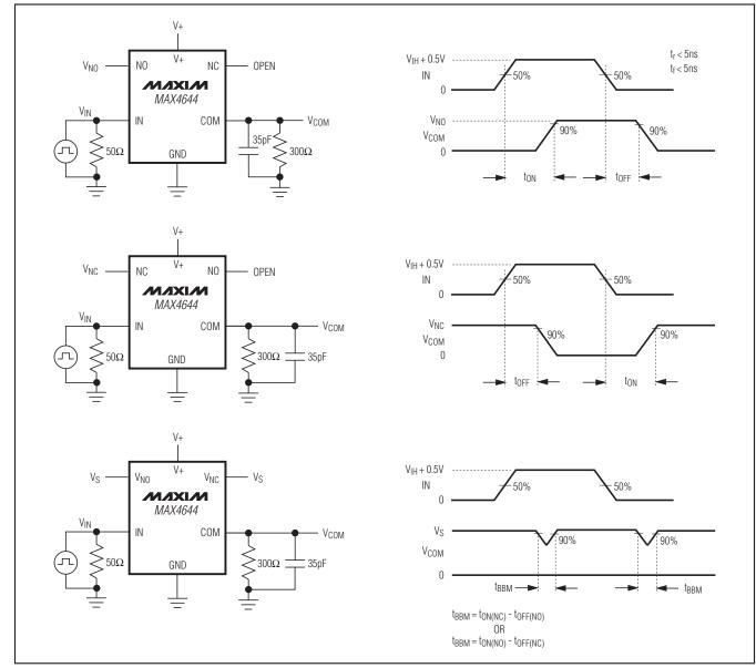
Figure 2. Switching Times
