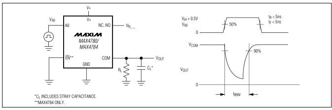
Figure 2. Break-Before-Make Interval
