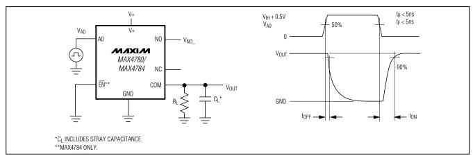
Figure 1. Turn-On and Turn-Off Times
