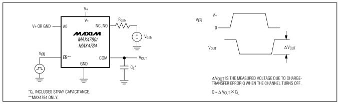
Figure 3. Charge Injection
