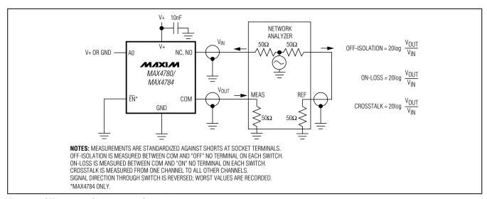
Figure 5. Off-Isolation, On-Loss, and Crosstalk
