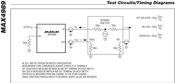
Figure 1. On-Loss, Off-Isolation, and Crosstalk
