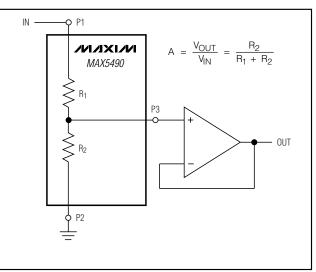
Figure 4. Attenuator with Buffer
