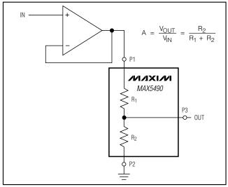
Figure 3. Buffered Attenuator
