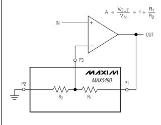
Figure 2. Noninverting Amplifier Configuration
