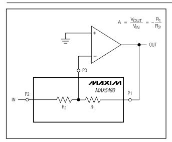
Figure 1. Inverting Amplifier Configuration
