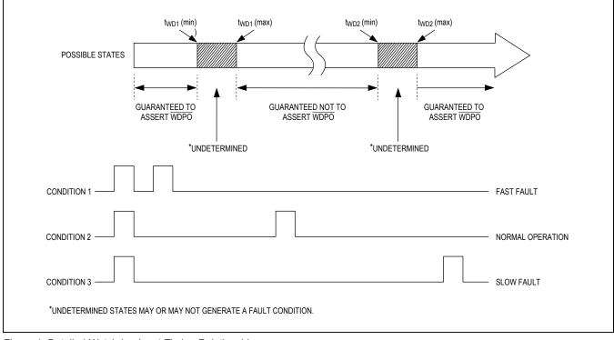
Figure 1. Detailed Watchdog Input Timing Relationship
