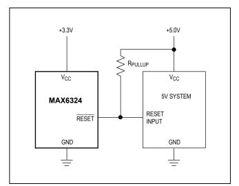
Figure 8. MAX6324 Open-Drain RESET Output Allows Use with Multiple Supplies
