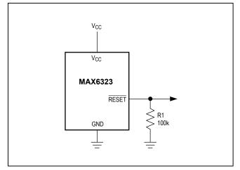
Figure 6. RESET Valid to V<sub>CC</sub> = Ground Circuit
