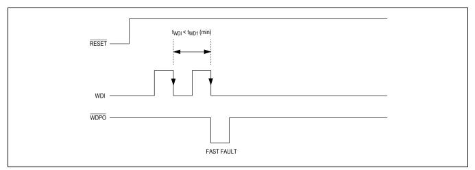
Figure 2. Fast Fault Timing
