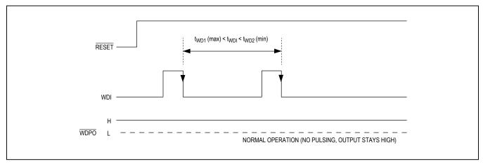
Figure 4. Normal Operation, WDPO Not Asserted
