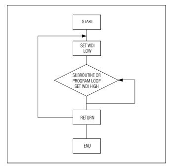
Figure 9. Watchdog Flow Diagram
