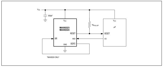
Figure 10. WDPO to MR Loopback Circuit
