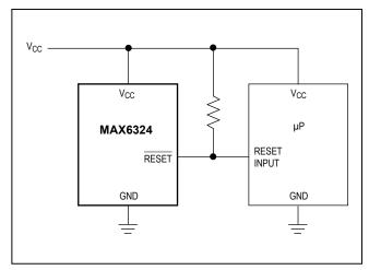
Figure 7. Interfacing to µPs with Bidirectional Reset Pins
