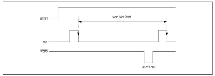
Figure 3. Slow Fault Timing
