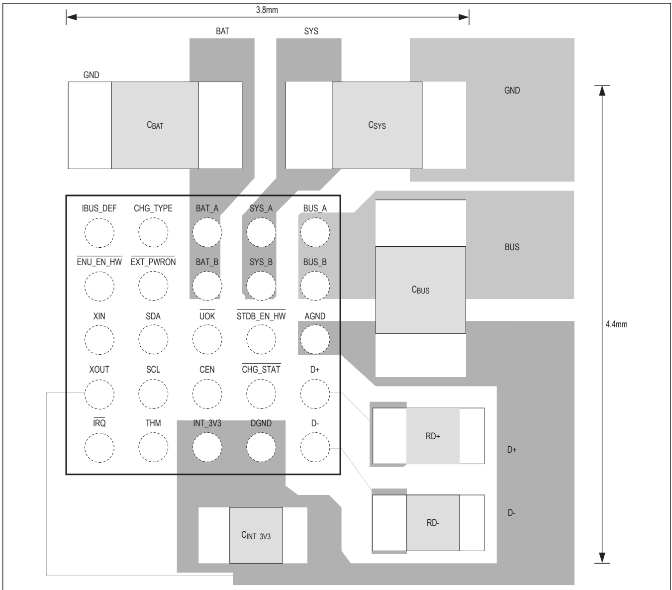
Figure 27. Recommended PCB Layout for Low Speed
