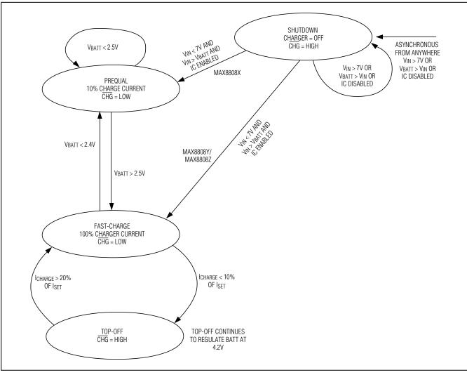
Figure 2. Charge-State Diagram
