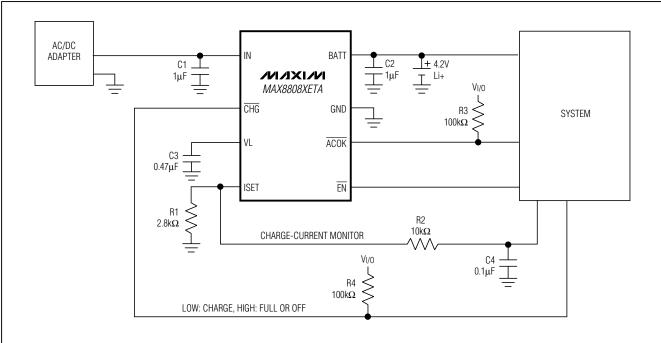
Figure 4. µP-Interfaced Li+ Battery Charger
