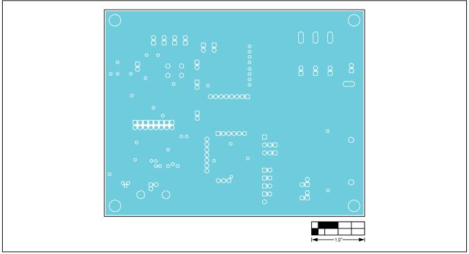
Figure 13. MAX9271 Coax EV Kit PCB Layout—Ground Layer 2
