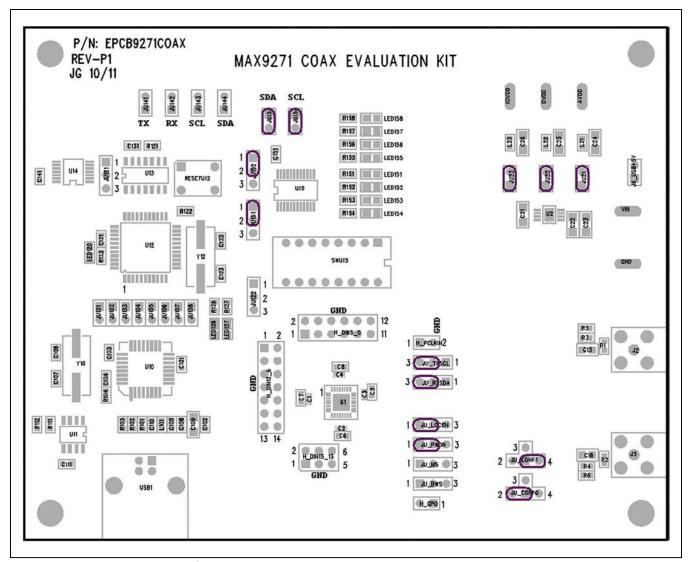
Figure 9. Initial Jumper Settings for I<sup>2</sup>C Mode
