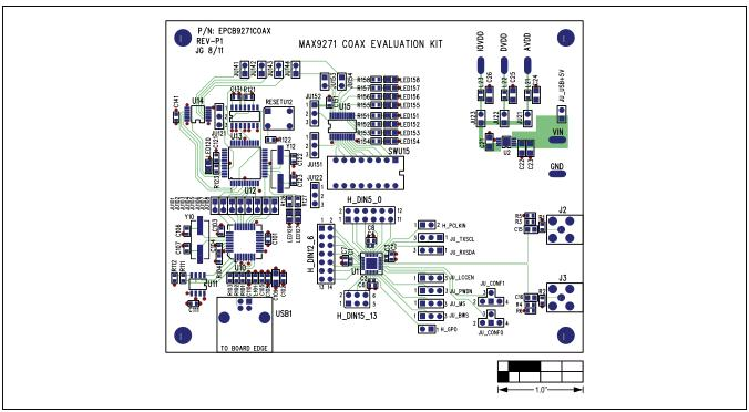
Figure 12. MAX9271 Coax EV Kit PCB Layout—Component Side
