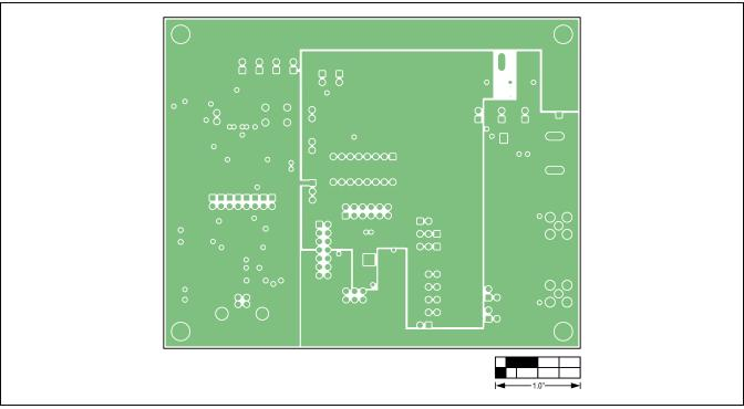
Figure 14. MAX9271 Coax EV Kit PCB Layout—Power Layer 3
