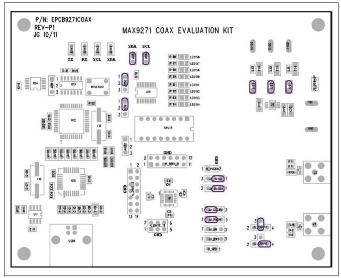
Figure 8. Initial Jumper Settings for UART Mode
