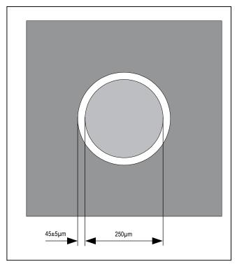
Figure 4. PCB Footprint Recommendation Diagram
