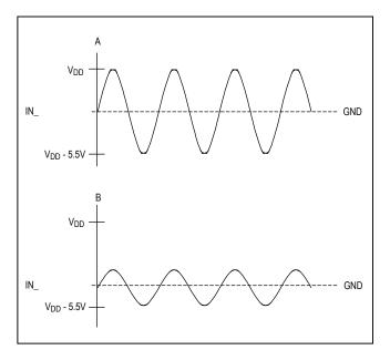
Figure 2. Proper Supply Selected for a Given Input Signal. A: Supply Voltage with a Large Signal; B: Supply Voltage with a Small Signal
