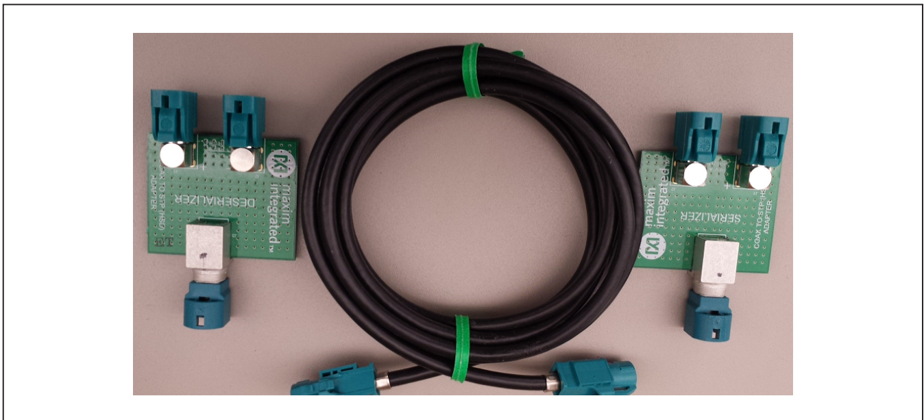
Figure 1. Photo of MAXCOAX2STP-HSD Adapter Kit Components
