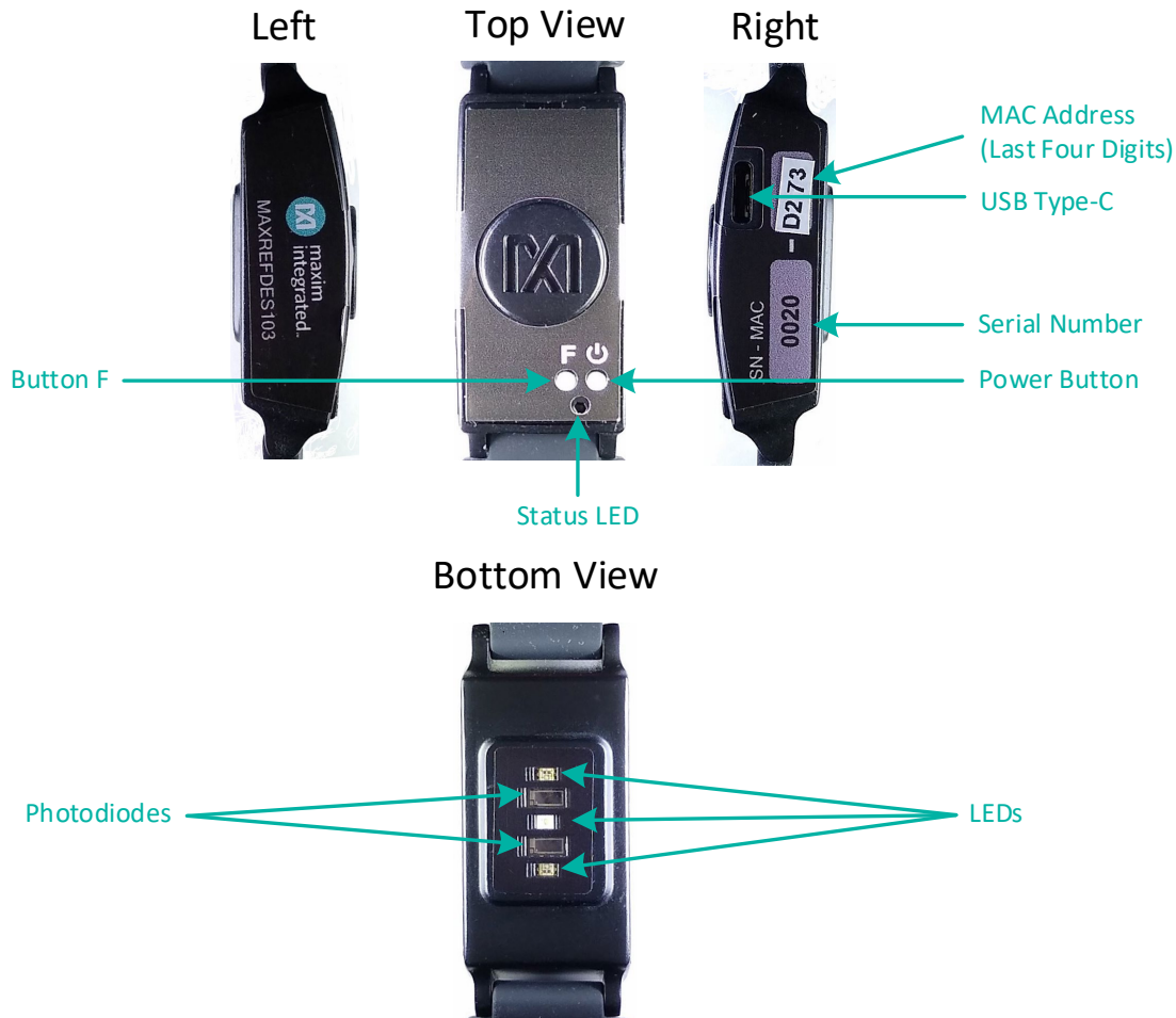
Figure 1. MAXREFDES103# wearable form factor in detail.
