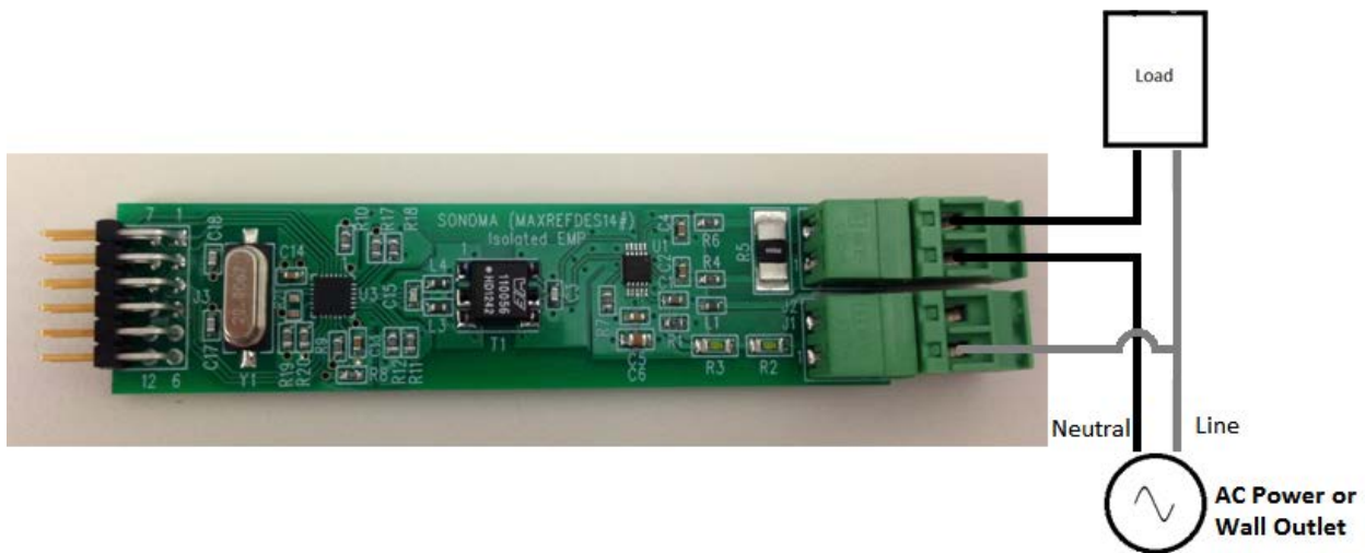
Figure 4. Sonoma Power and Load Connections
