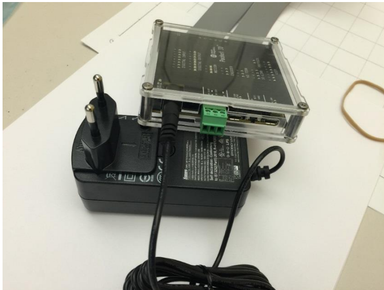
Figure 10. Pocket IO with Power Supply Connected.
