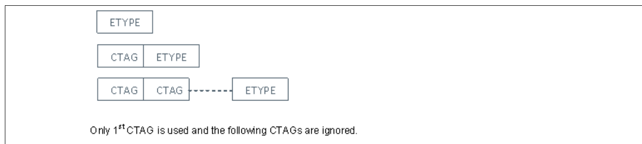
Figure 27 Supported Frame Formats when STAG is disabled
