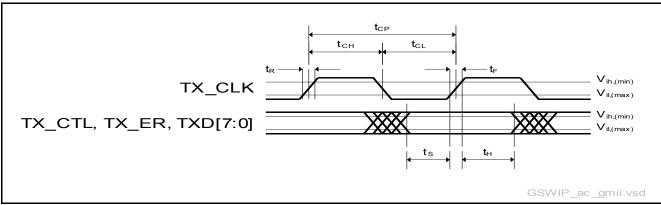
Figure 50 Transmit Timing Diagram of the GMII
