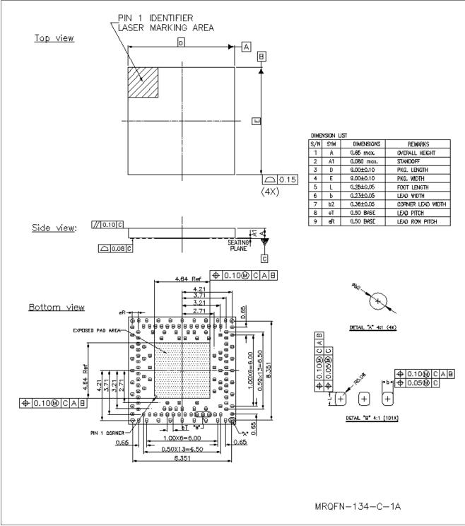
Figure 54 PG-MRQFN-134-C-1A 9 mm x 9 mm Package Outline
