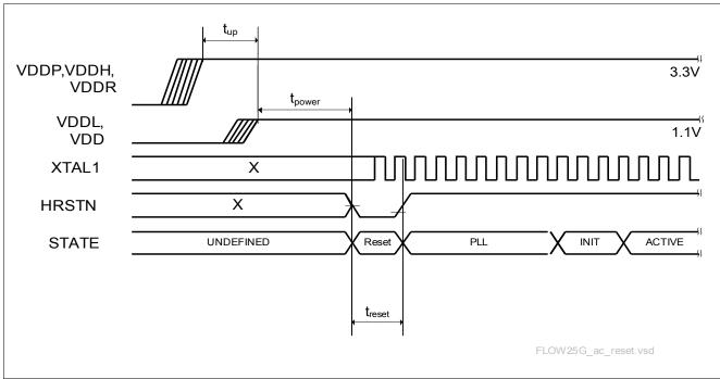
Figure 47 Timing Diagram for the GSW150 Reset Sequence
