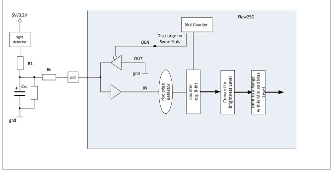
Figure 16 Light Sensing System
