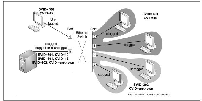
Figure 30 Double Tag and Port based VLAN Example
