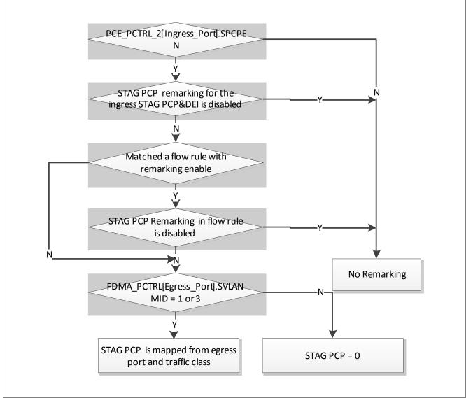
Figure 35 STAG PCP Remarking Flow Diagram
