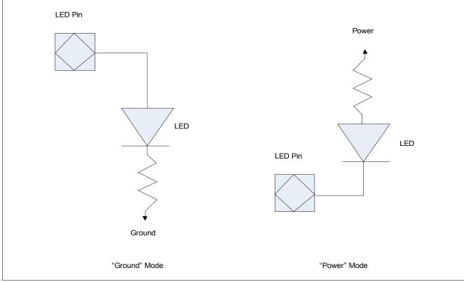
Figure 11 LED Display Mode
