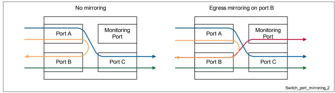
Figure 42 Port Mirroring Examples – Egress Monitoring
