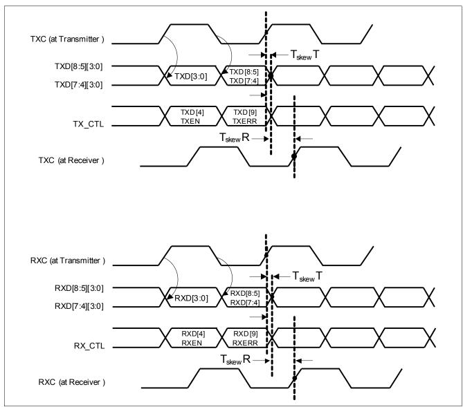
Figure 52 Timing Diagram of the RGMII
