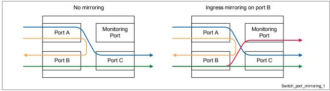
Figure 41 Port Mirroring Examples – Ingress Monitoring
