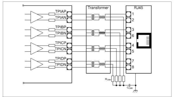
Figure 19 Twisted-Pair Interface of GPHY IP Including Transformer and RJ45 Plug
