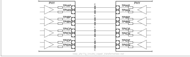
Figure 20 External Circuitry for the Transformerless Ethernet Application
