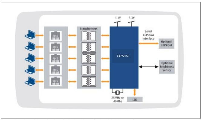
Figure 1 Standalone Desktop Switch with an Optional Brightness Sensor
