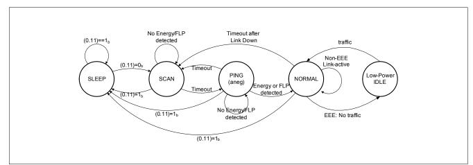
Figure 21 State Diagram for Power-Down Mode Management
