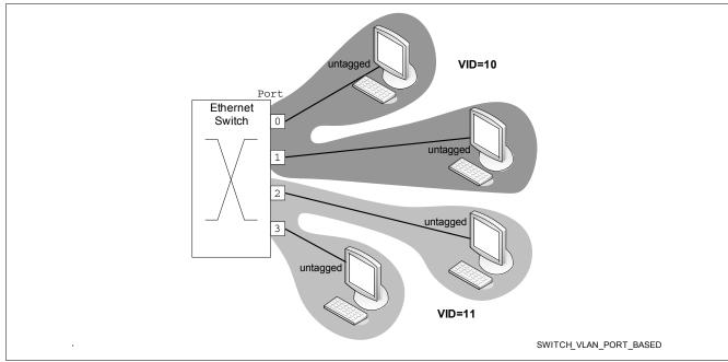
Figure 28 Port-based VLAN Example
