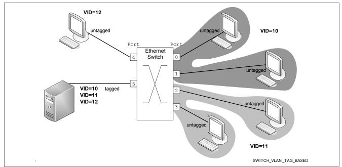
Figure 29 Tag-based VLAN Example
