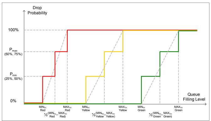
Figure 39 Drop Precedence Thresholds
