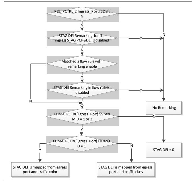
Figure 36 STAG DEI Remarking Flow Diagram
