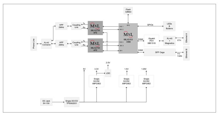
Figure 2: Wave-2 DCP962P Adapter Block Diagram
