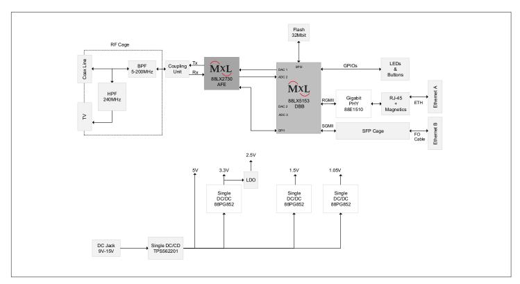
Figure 1: Wave-2 DCP962C Adapter Block Diagram
