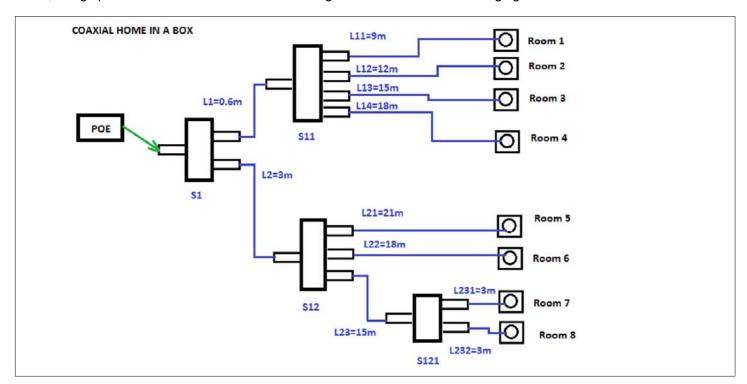
Figure 8: Coax "Home In A Box" Test Bench
