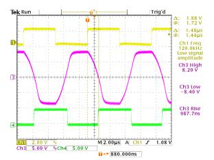
Figure 8: SP211E and SP213E Transmitter Output @ 240kbps $R_1 = 3k\Omega$ ,  $C_1 = 1000pF$
