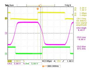
Figure 6: SP211E and SP213E Transmitter Output @ 120kbps  $R_1 = 3k\Omega$ ,  $C_1 = 1000pF$
