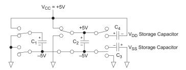
Figure 8: Charge Pump - Phase 3
