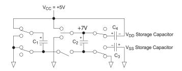
Figure 9: Charge Pump - Phase 4
