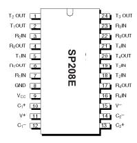
Figure 3: SP208E Pin Configuration
