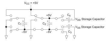
Figure 6: Charge Pump - Phase 1
