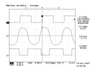
Figure 5: SP208E Transmitter Output @ 240kbps  $R_1 = 3k\Omega$ ,  $C_1 = 2500pF$
