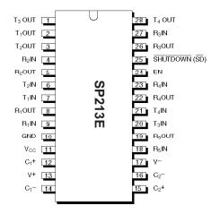
Figure 5: SP213E Pin Configuration
