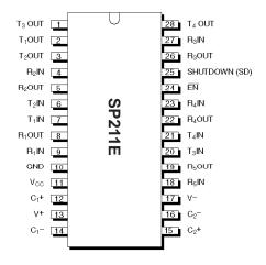
Figure 4: SP211E Pin Configuration
