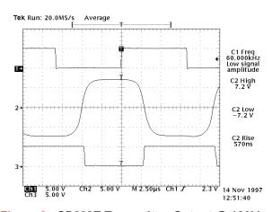
Figure 3: SP208E Transmitter Output @ 120kbps  $R_{L} = 3k\Omega$ ,  $C_{L} = 2500pF$
