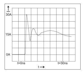
Figure 14: ESD Test Waveform for IEC61000-4-2
