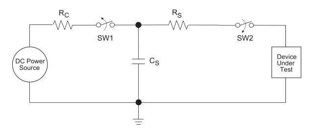
Figure 12: ESD Test Circuit for Human Body Model
