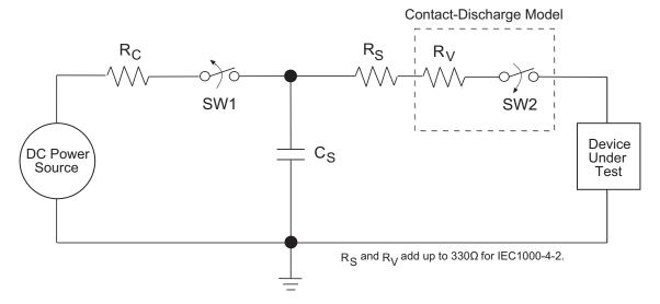
Figure 13: ESD Test Circuit for IEC61000-4-2
