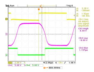
Figure 7: SP211E and SP213E Transmitter Output @ 120kbps  $R_L = 3k\Omega$ ,  $C_L = 2500pF$
