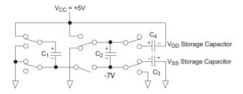
Figure 7: Charge Pump - Phase 2
