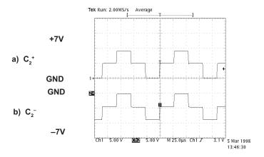
Figure 10: Typical Waveforms Seen on Capacitor C2
