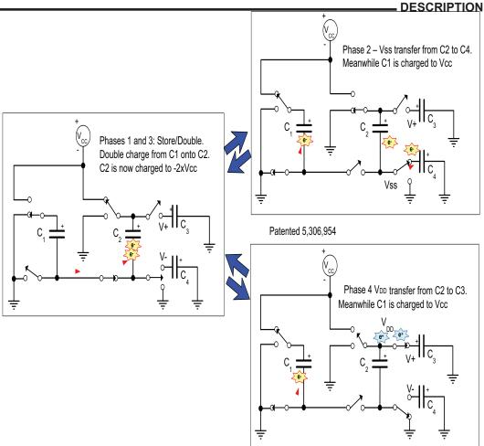
Figure 1. Charge pump phases
