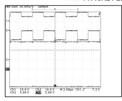
Figure 3, SP232E Charge pump waveformsno load (1 = C1+, 2 = C2+, 3 = V+, 4 = V-).
