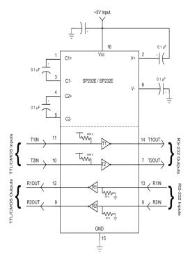
Figure 7, SP202E and SP232E Typical Application circuit
