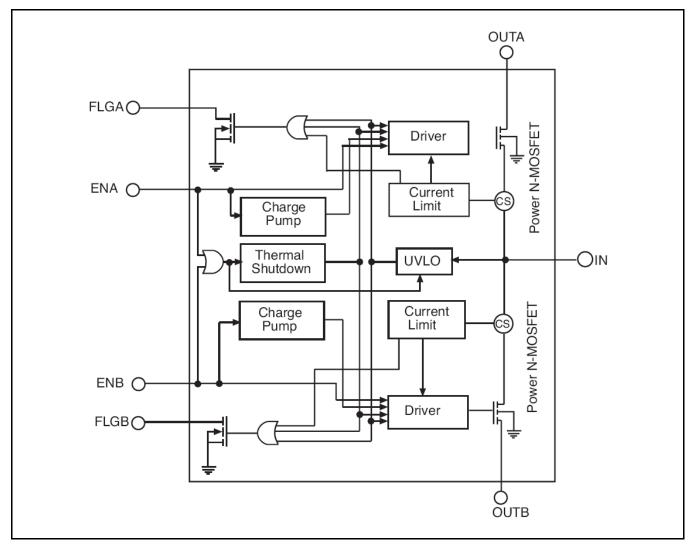
Fig. 2: SP2526A Block Diagram
