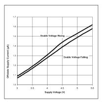
Fig. 11: Control Threshold vs Supply Voltage
