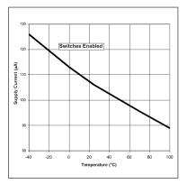
Fig. 8: On-state Supply Current vs Temperature
