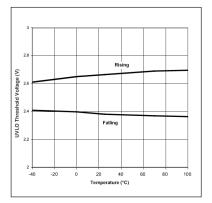
Fig. 6: UVLO Threshold vs Temperature
