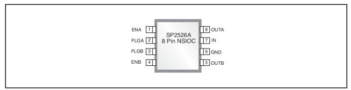
Fig. 3: SP2526A Pin Assignment
