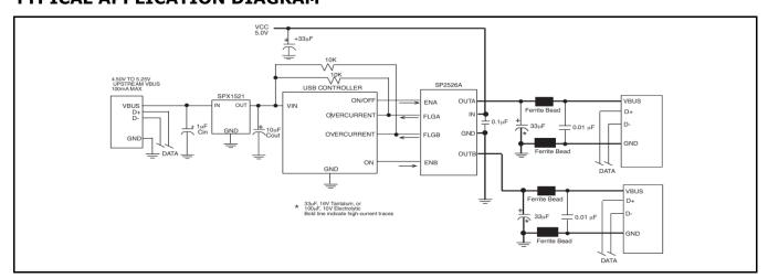
Fig. 1: SP2526A Application Diagram - Two Port Self Powered Hub
