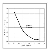
Fig. 4: Output On-Resistance vs Supply Voltage
