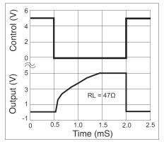
Fig. 12: Turn-on/Turn-off Characteristics
