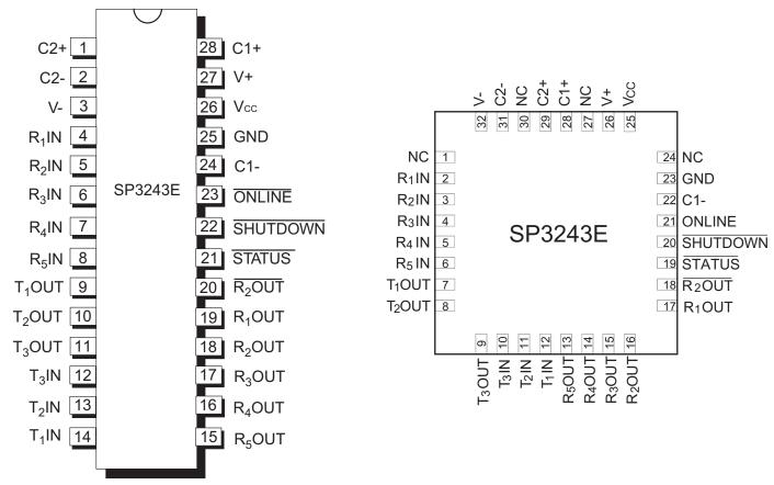
Figure 8: SP3243E Pinout (Top View) SSOP / TSSOP
