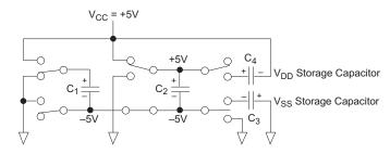
Figure 15: Charge Pump — Phase 1
