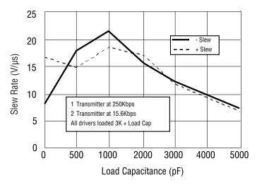
Figure 7: Slew Rate vs. Load Capacitance
