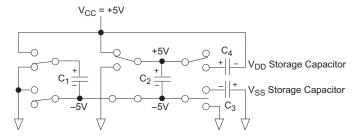
Figure 17: Charge Pump — Phase 3
