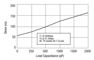
Figure 1: Transmitter Skew vs. Load Capacitance
