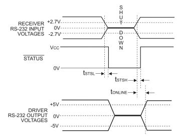
Figure 19: AUTO ON-LINE Timing Waveforms
