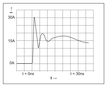
Figure 27: ESD Test Waveform for IEC61000-4-2
