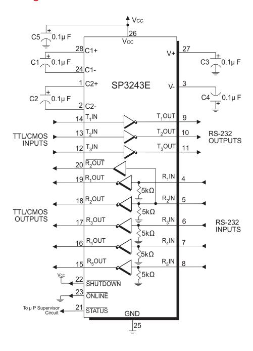
Figure 10: SP3243E Typical Operating Circuit
