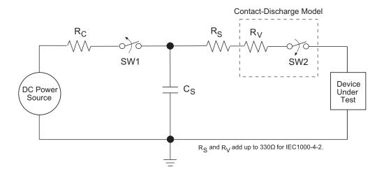
Figure 26: ESD Test Circuit for IEC61000-4-2
