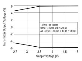
Figure 2: Transmitter Output Voltage vs. Supply Voltage for the SP3243EU
