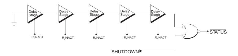
Figure 24: Stage II of AUTO ON-LINE Circuitry
