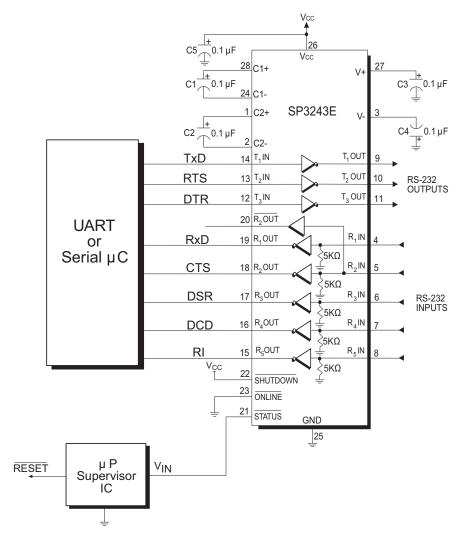
Figure 11: Interface Circuitry Controlled by Microprocessor Supervisory Circuit
