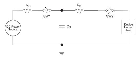
Figure 25: ESD Test Circuit for Human Body Model
