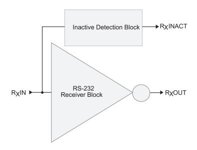
Figure 23: Stage I of AUTO ON-LINE Circuitry
