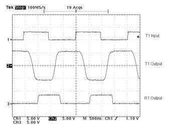
Figure 13: Loopback Test Results at 1Mbps
