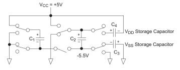
Figure 16: Charge Pump — Phase 2
