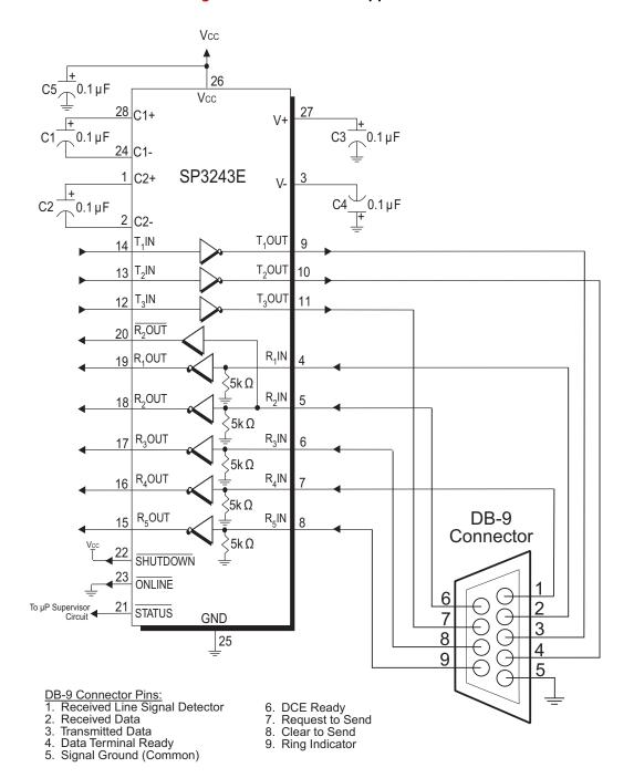
Figure 22: Attaching SP3243E to a DB-9 Connector
