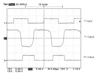
Figure 14: Loopback Test Results at 250kbps
