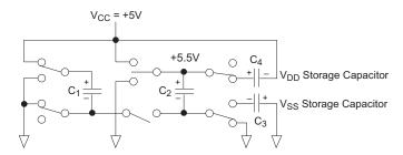
Figure 18: Charge Pump — Phase 4
