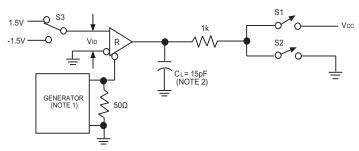
Figure 7: Receiver Enable and Disable Timing Circuit
