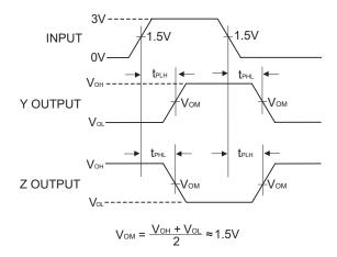
Figure 9: Driver Propagation Delay Waveforms
