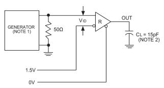
Figure 6: Receiver Propagation Delay Test Circuit
