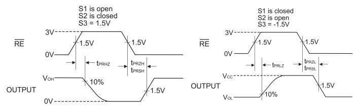
Figure 13: Receiver Enable and Disable Waveforms
