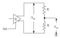
Figure 1: Driver DC Test Load Circuit
