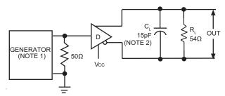
Figure 2: Driver Propagation Delay Test Circuit
