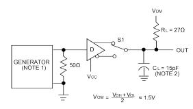
Figure 4: Driver Propagation Delay Test Circuit
