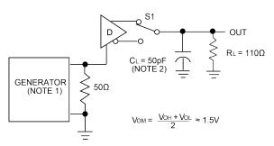
Figure 6: Driver Enable and Disable Timing Circuit, Output High
