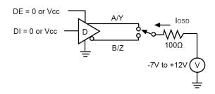
Figure 10: Driver Short Circuit Current Limit Test
