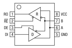
Figure 2: SP3494 Pinout (Top View)
