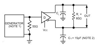
Figure 5: Driver Differential Output Delay and Transition Time Circuit
