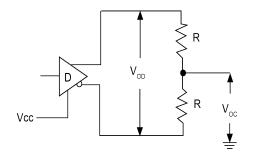
Figure 3: Driver DC Test Load Circuit
