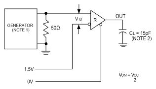
Figure 8: Receiver Propagation Delay Test Circuit
