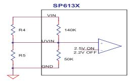
Figure 4- Internal and external bias of UVIN
