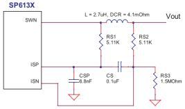
Figure 3- Over-current detection circuit for IMAX < {60mV/DCR}
