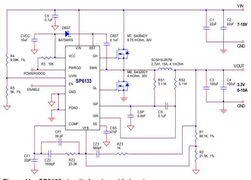
Figure 11: SP6133 circuit showing wide input range
