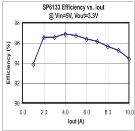
Figure 9: Efficiency vs. Iout, Vin = 5V
