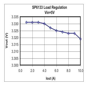
Figure 10: Load Regulation, 5V
