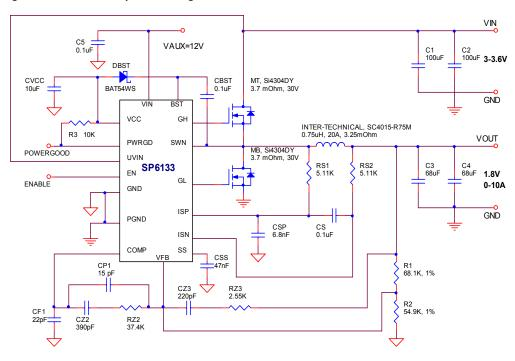
Figure 14. SP6133: 3.3V Input Buck Regulator with auxiliary 12V bias
