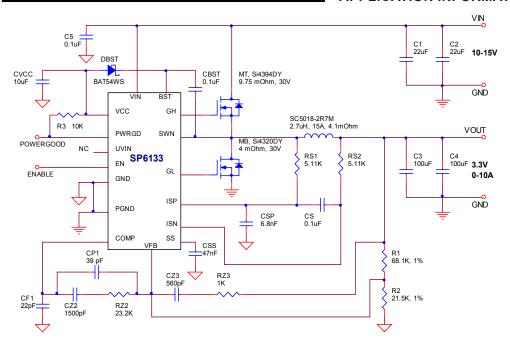
Figure 15. SP6133: 10-15V Input Buck Regulator
