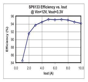
Figure 7: Efficiency vs. IOUT, VIN = 12V
