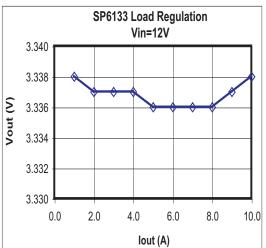
Figure 8: Load Regulation, 12V
