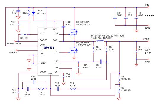
Figure 13. SP6133: 5V Input Buck Regulator
