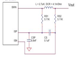
Figure 1: Over-current detection circuit
