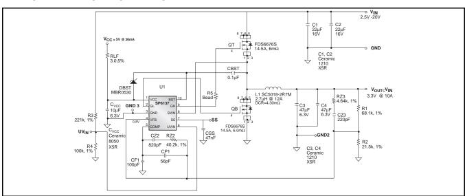
Fig. 1: SP6137 Application Diagram
