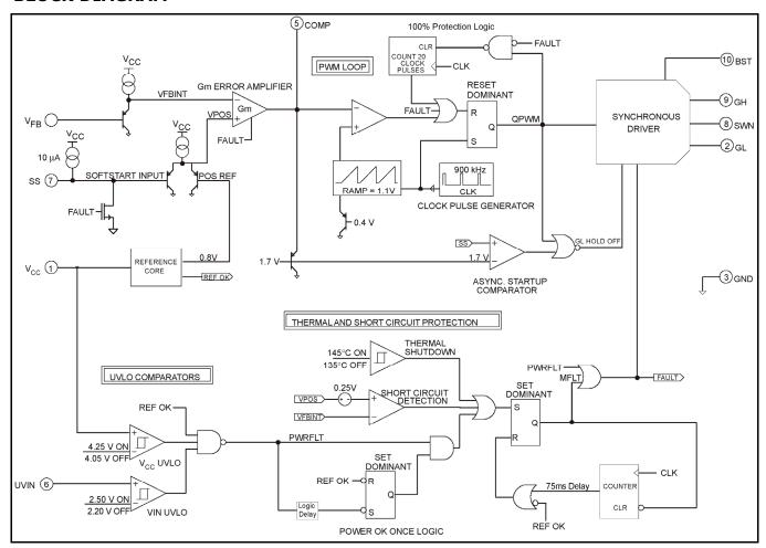
Fig. 2:SP6137 Block Diagram
