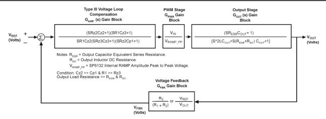
SP6137 Voltage Mode Control Loop with Loop Dynamic
