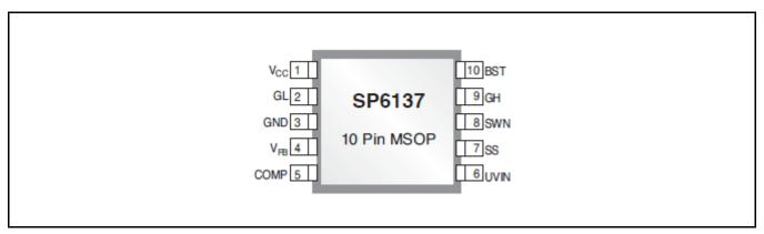
Fig. 3: SP6137 Pin Assignment
