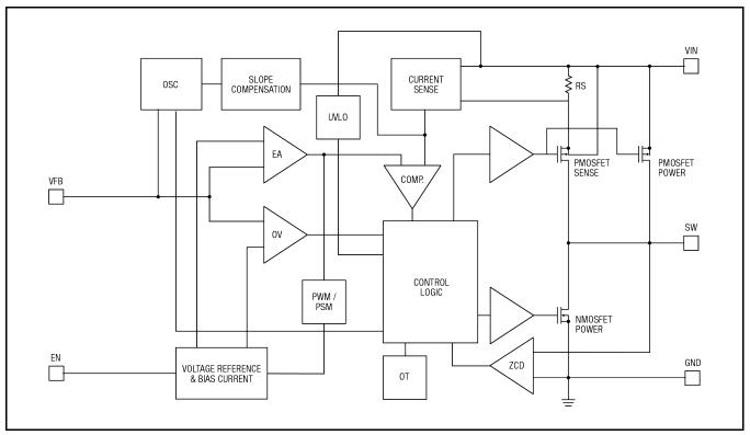
Fig. 2: SP6669 Block Diagram
