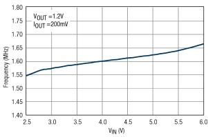
Fig. 5: Oscillator Frequency vs. Input Voltage
