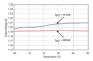
Fig. 9: Output Voltage vs Temperature
