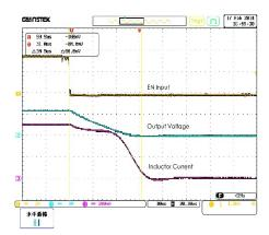
Fig. 17: Power-OFF from EN Pin
