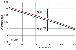
Fig. 7: EN Pin Threshold vs. Temperature
