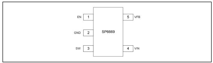
Fig. 3: SP6669 Pin Assignment
