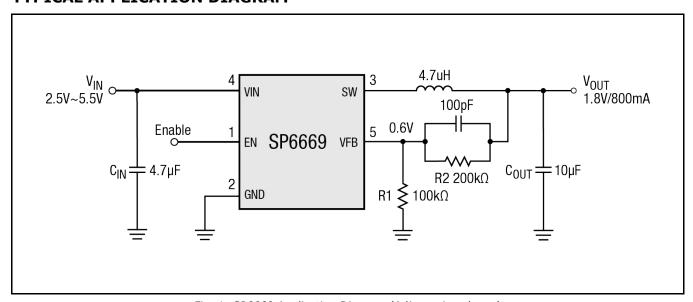
Fig. 1: SP6669 Application Diagram (Adj. version shown)
