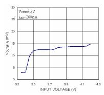
Fig. 20: VOUT Ripple Voltage for VIN decreasing close to  $V_{\text{OUT}}$
