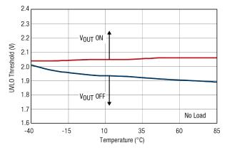
Fig. 8: UVLO Threshold vs. Temperature
