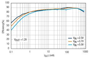
Fig. 4: Efficiency vs Output Current  $V_{OUT} = 1.2V$
