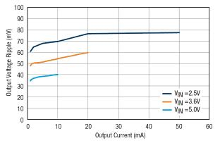
Fig. 15: Output Voltage Ripple vs Output Current
