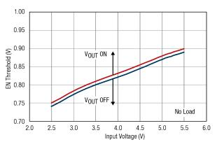
Fig. 6: EN Pin Threshold vs. Input Voltage
